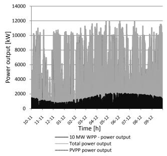
Fig. 5 One year data of output power from the hybrid system for Case II - hourly values
