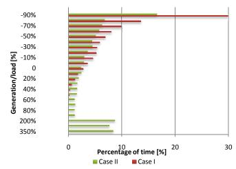
Fig. 8 Hybrid system electricity generation relative to consumption - one year data
