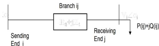
Fig.3 Electrical equivalent of one branch
