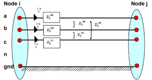
Fig. 1 – Three phase four wire line model
