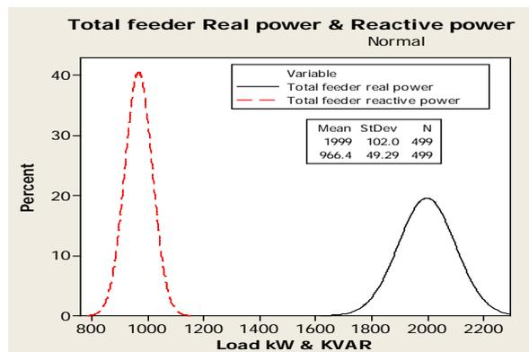
Fig. 6. Distribution of Feeder Real and Reactive power
