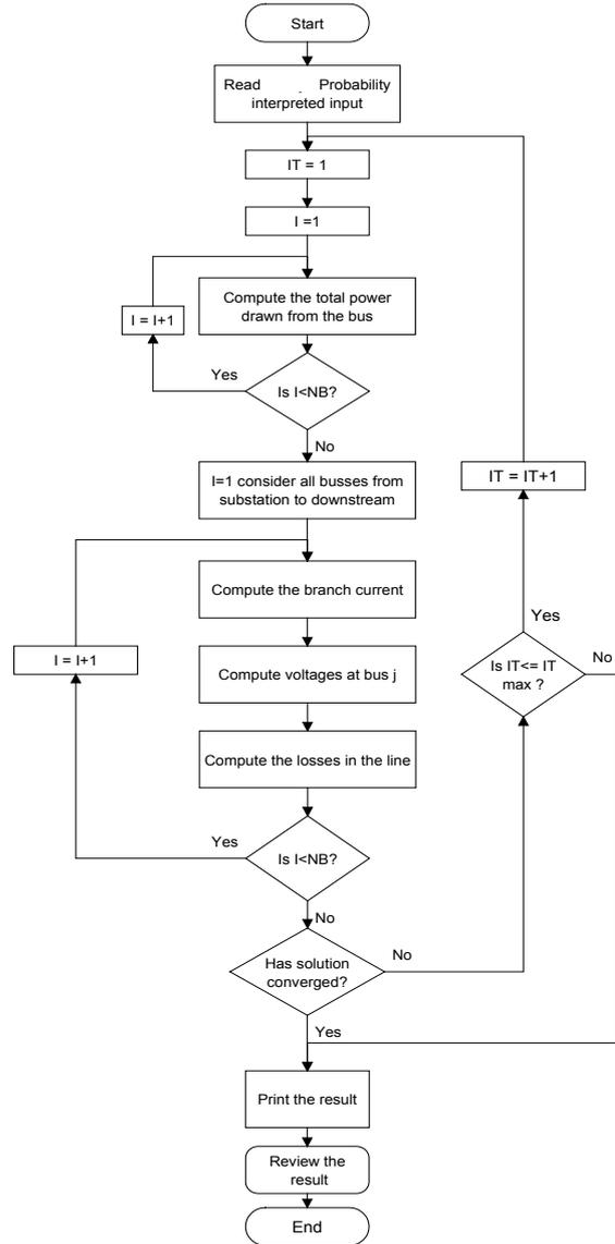
Fig. 2. Typical monte-carlo load flow calculation chart used with probability interpreted inputs
