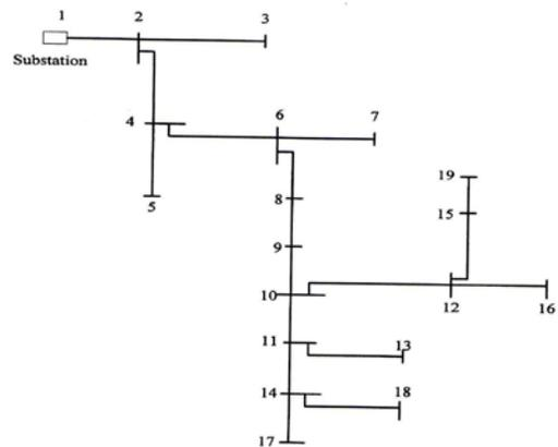
Fig. 5. Shows a practical 19 bus distribution feeder used for the modelling and simulation purpose.
