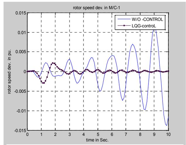
Fig. 10: Rotor speed dev. Response due to 0.1 load disturbance with and without LQG control of M/C-1.
