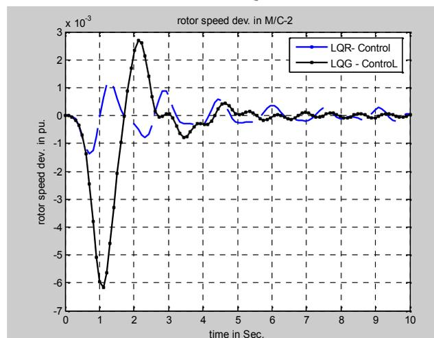
Fig.12: Rotor speed dev. Response due to 0.1 load disturbance with LQG and LQR controllers of M/C-2.
