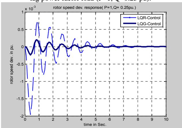
Fig. 7: Rotor speed dev. Response due to 0.1 load disturbance with LQG compared with LQR controller at lag power factor load (P=1, Q=0.25 pu).
