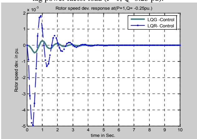
Fig. 8: Rotor speed dev. Response due to 0.1 load disturbance with LQG compared with LQR controller at lead power factor load (P=1, Q= -0.25 pu).
