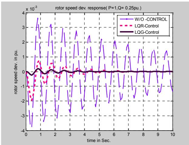
Fig.6: Rotor speed dev. Response due to 0.1 load disturbance with and without LQG and LQR controllers at lag power factor load (P=1, Q=0.25 pu).
