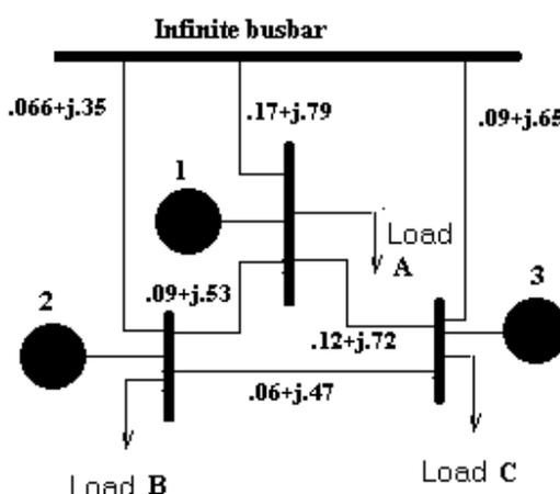
Fig.2: Three machine-infinite bus system.
