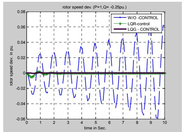
Fig. 9: Rotor speed dev. Response due to 0.1 load disturbance with and without LQG and LQR controllers at lead power factor load (P=1, Q= -0.25 pu).
