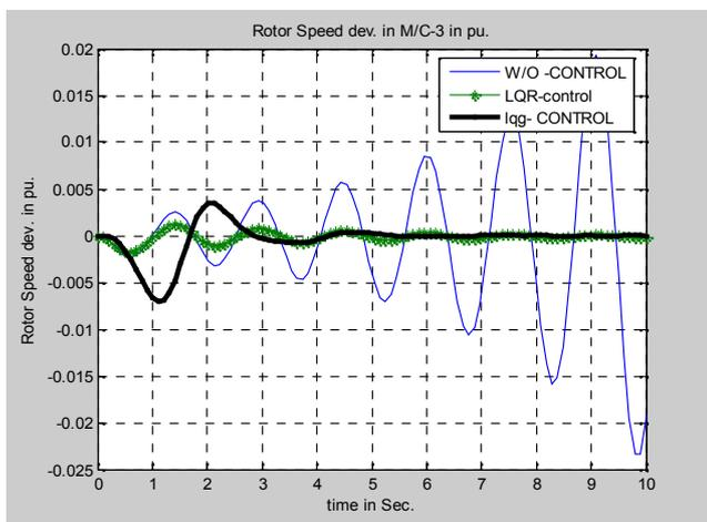
Fig. 14: Rotor speed dev. Response due to 0.1 load disturbance with and without LOG and LQR control of M/C-3.
