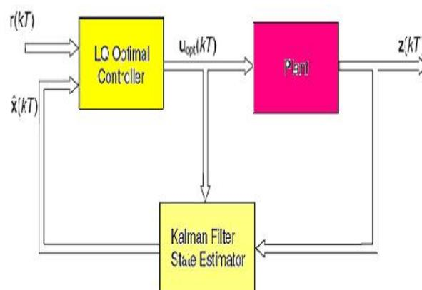
Fig. 3: Linear Quadratic Gaussian (LQG) control system.
