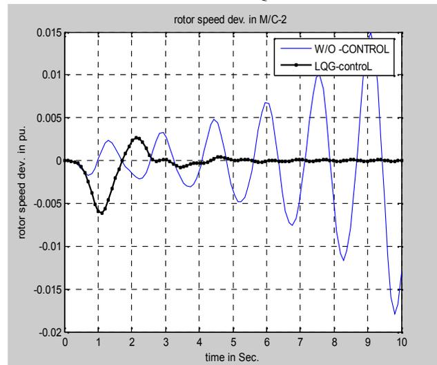
Fig.11: Rotor speed dev. Response due to 0.1 load disturbance with and without LQG control of M/C-2.
