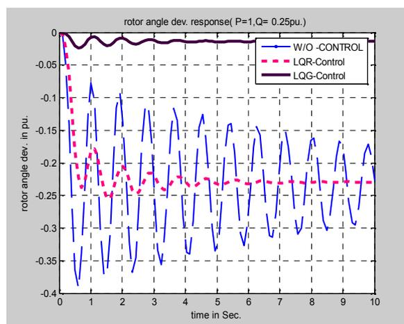
Fig.5: Rotor angle dev. Response due to 0.1 load disturbance with and without LQG and LQR controllers at lag power factor load (P=1, Q=0.25 pu).
