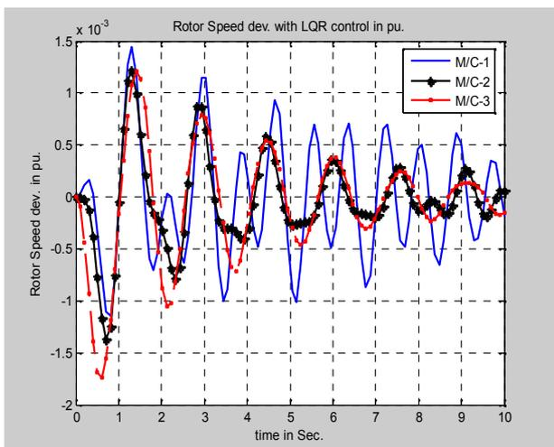
Fig. 15: Rotor speed dev. Response due to 0.1 pu load disturbance with LQR control for three machines.
