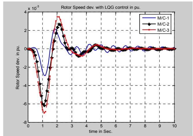
Fig. 16: Rotor speed dev. Response due to 0.1 pu load disturbance with LQG control for three machines.
