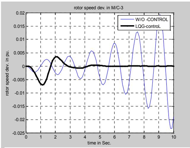
Fig. 13: Rotor speed dev. Response due to 0.1 load disturbance with and without LQG control of M/C-3.
