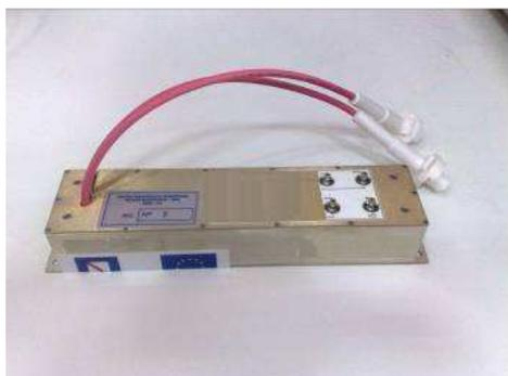
Fig. 14 - Photo of the voltage divider of the RVT.
