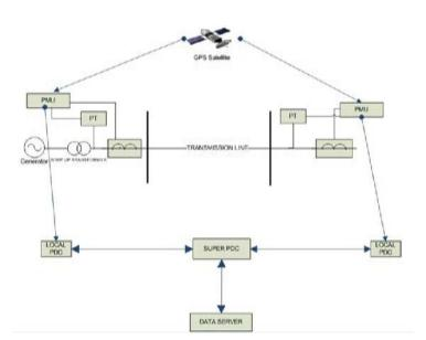
Figure 1.1: Block diagram of WAMPAC
