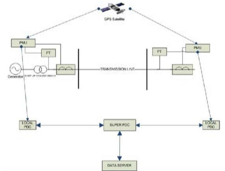
Figure 1.1: Block diagram of WAMPAC
