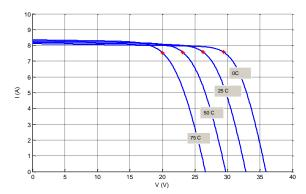
Fig. 5 Current VS Voltage Characteristic curve  $(G=1000W/m^2)$
