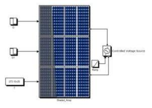
Fig. 8 Simulink Block of partially shaded Array .
