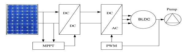
Fig. 1 Block diagram of the BLDC water pumping system
