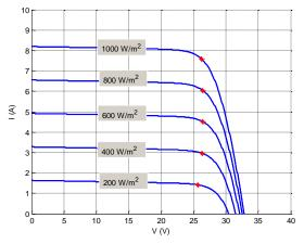
Fig. 3 Current VS Voltage Characteristic (T=25°c)
