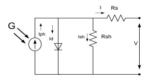
Fig. 2 Block of equivalent circuit of PV cell
