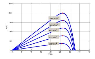
Fig. 4 Power VS Voltage Characteristic curve (T=25°c)
