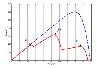
Fig. 10 Comparison between P-V curve uniform and partially shaded PV array
