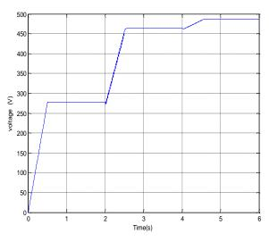
Fig. 18 boost converter output voltage
