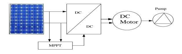
Fig. 15 Block diagram of the D.C water pump
