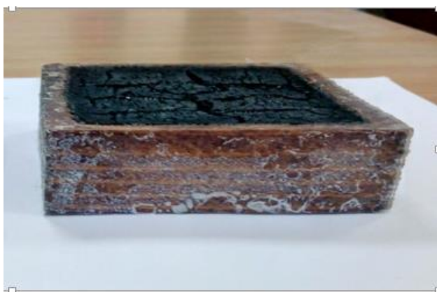
Fig. 3 Painted Beech wood under an irradiance of 25 kW/m 2
