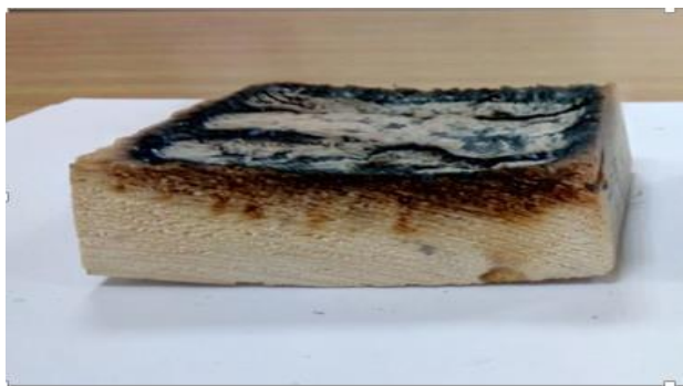
Fig. 2 Unpainted Beech wood under an irradiance of 25 kW/m 2
