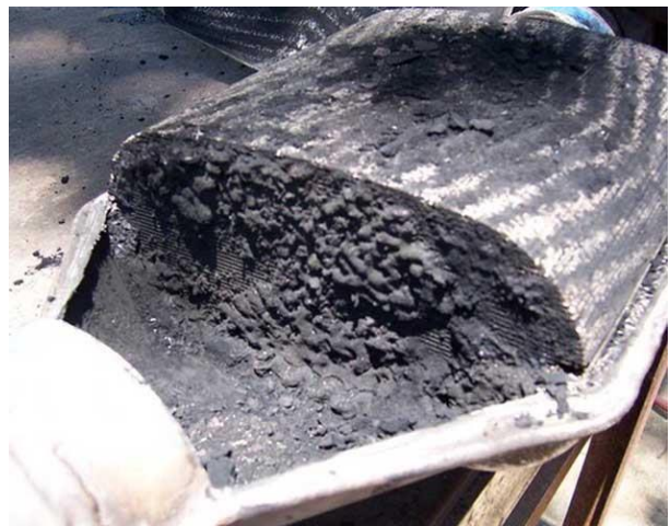
Fig 2: Blocked Diesel Particulate Filter[1]
