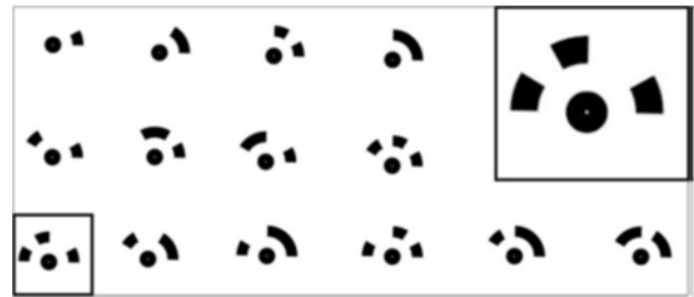
Fig. 1. Pattern of external camera calibration target code
