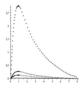
Fig.6. The function y(x), obtained at a fixed value of the Poisson's ratio  $\sigma = 0.01$  and at different initial conditions. The solid curve, enlarged tenfold corresponds to y'(0) = 0.01, quadrangles - y'(0) = 0.5, crosses - y'(0) = 1, asterisks - y'(0) = 10.
