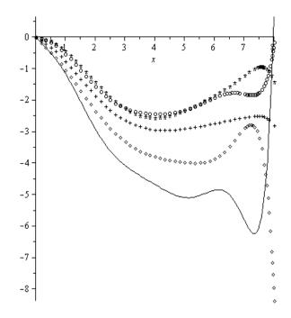
Fig.9. The dependence  $u_z(x)$ , constructed under a constant condition y'(0) = 1 for different values of the Poisson's ratio  $\sigma$ . The solid curve corresponds to  $\sigma = 0.1$ , quadrangles -  $\sigma = 0.2$ , crosses -  $\sigma = 0.3$ , circles -  $\sigma = 0.4$ , asterisks -  $\sigma = 0.45$ .
