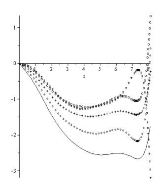
Fig.8. The dependence  $u_z(x)$ , constructed under a constant condition y'(0) = 0.5 for the different values of the Poisson's ratio  $\sigma$ . The solid curve corresponds to  $\sigma = 0.1$ , quadrangles -  $\sigma = 0.2$ , crosses -  $\sigma = 0.3$ , circles -  $\sigma = 0.4$ , asterisks -  $\sigma = 0.45$ .
