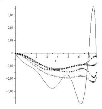
Fig.7. The dependence  $u_z(x)$ , constructed under a constant condition y'(0) = 0.01 for different values of the Poisson's ratio  $\sigma$ . The solid curve corresponds to  $\sigma = 0.1$ , quadrangles -  $\sigma = 0.2$ , crosses -  $\sigma = 0.3$ , circles -  $\sigma = 0.4$ , asterisks -  $\sigma = 0.45$ .
