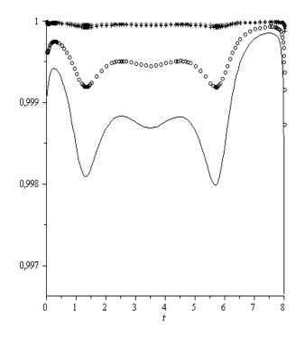
Fig.14. The dependencies  $\varepsilon(\lambda)$ , obtained when a cylindrical rod hits different materials moving at a speed of 30 m / s after contact with the steel medium. The solid curve corresponds to  $\sigma = 0.1$  (concrete), quadrangles -  $\sigma = 0.2$  (cast iron), crosses -  $\sigma = 0.3$  (cuprum), circles -  $\sigma = 0.4$  (plumbum).
