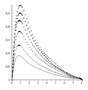
Fig.1. The function y(x), obtained for the fixed initial condition y'(0) = 1 and at different coefficient values of the Poisson's ratio  $\sigma$ . All the curves are in accord with theoretical meanings of Poisson's coefficient (from now on). Solid curve conforms with  $\sigma = 0.45$ , quadrangles -  $\sigma = 0.4$ , crosses-  $\sigma = 0.3$ , circles -  $\sigma = 0.2$ , black boxes - $\sigma = 0.1$ , asterisks-  $\sigma = 0.01$ .
