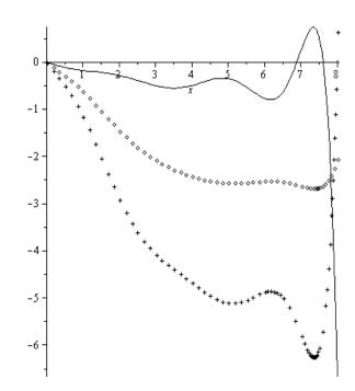
Fig.12. The dependence  $u_z(x)$ , constructed under constant value of the Poisson's ratio  $\sigma = 0.1$  for different initial conditions. The solid curve, enlarged tenfold corresponds to y'(0) = 0.01, circlesy'(0) = 0.5, crosses - y'(0) = 1.
