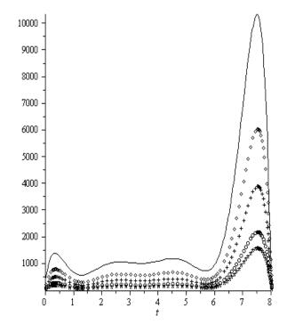
Fig. 16. The dependence  $S_{\sigma}(C,\lambda)$ , obtained for different varies of the Poisson's ratio. The solid curve corresponds to  $\sigma = 0.1$  (concrete), quadrangles -  $\sigma = 0.2$  (cast iron), crosses -  $\sigma = 0.3$  (cuprum), circles -  $\sigma = 0.4$  (plumbum), asterisks -  $\sigma = 0.45$ (caoutchuc). The initial condition for function y(x)here y'(0) = 0.5.
