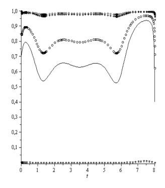
Fig. 15. The dependencies  $\varepsilon(\lambda)$ , obtained when a cylindrical rod hit different materials moving at a speed of 10 m / s after contact with the rubber medium. The solid curve corresponds to  $\sigma = 0.1$
