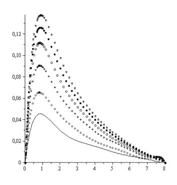
Fig.2. The function y(x), obtained for an fixed initial condition y'(0) = 0.5 and at different coefficient values of the Poisson's ratio  $\sigma$ . Solid curve conforms with  $\sigma = 0.45$ , quadrangles - $\sigma = 0.4$ , crosses -  $\sigma = 0.3$ , circles -  $\sigma = 0.2$ , black boxes -  $\sigma = 0.1$ , asterisks -  $\sigma = 0.01$ .
