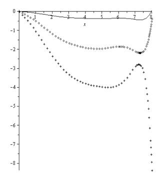
Fig.11. The dependence  $u_z(x)$ , constructed under constant value of the Poisson's ratio  $\sigma = 0.2$  for different initial conditions. The solid curve, enlarged tenfold corresponds to y'(0) = 0.01, circles - y'(0) = 0.5, crosses - y'(0) = 1.
