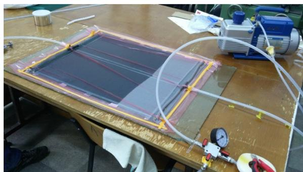
Fig. 3 Lower and upper panels VARTM assembly
