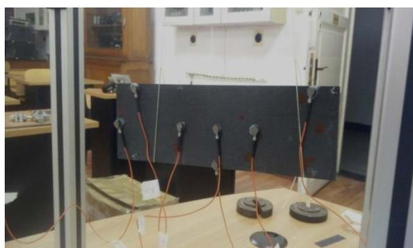
Fig. 5 Instrumentation of the 0° laminated plate for OMA
