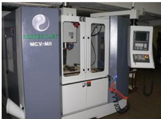
Fig.3. Machine tool applied for outer boring (PERFECT-JET MCV-M8)
