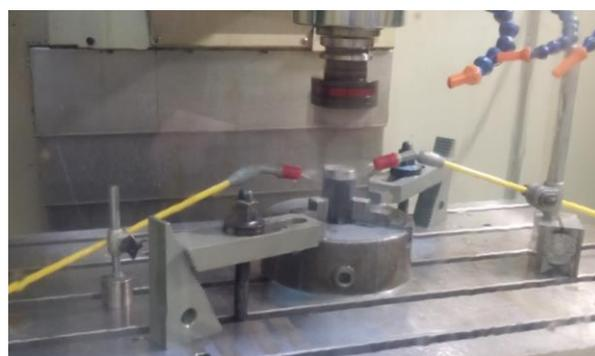
Fig.6. Outer boring during machining
