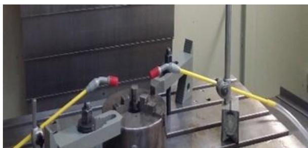
Fig.5. The position of the spraying heads relative to the workpiece in the machining area before cutting
