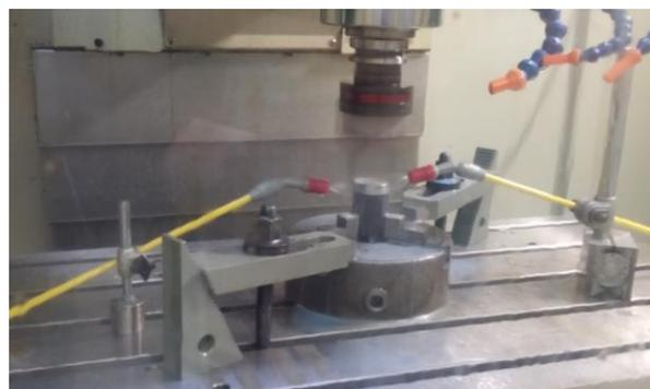
Fig.6. Outer boring during machining
