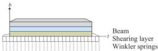
Fig.2 Pasternak model for the two-parameter foundation
