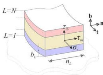
Fig.1 The stresses in the Frenet Coordinate System (N: Total number of layers)
