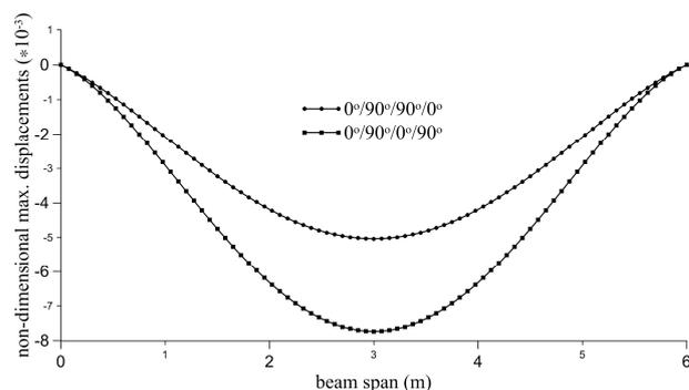
**Fig.3** The variation of non-dimensional maximum displacements of laminated composite straight beam with C-C boundary condition
