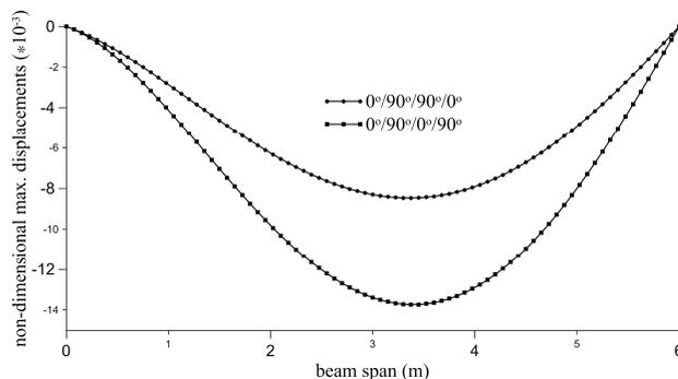
**Fig.4** The variation of non-dimensional maximum displacements of laminated composite straight beam with for C-S boundary condition
