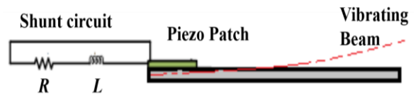
Fig. 4 Schematic of passive shunt dampers
