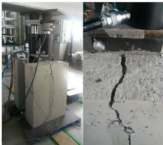
Figure 10: Failure of the test specimen V9
