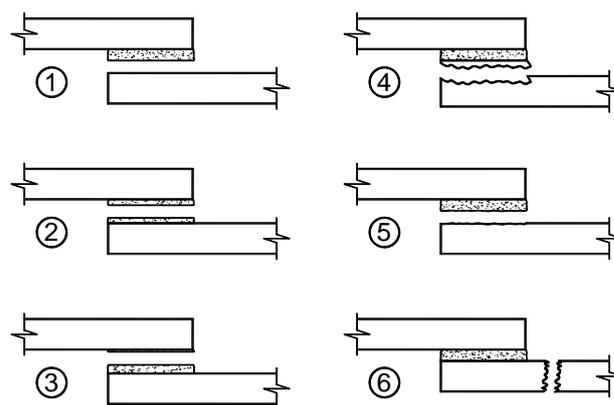
Fig. 9 Modes of failure in case of adhesively bonded joints of (G)FRP members
