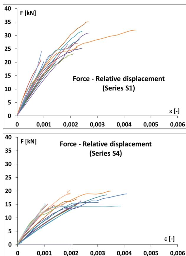
Fig. 8 Force to relative displacements relationships in case of series of specimens S1 and S4
