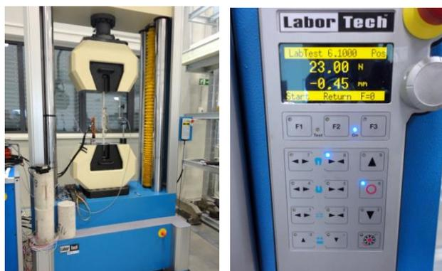
Fig. 3 Testing machine used for loading tests of the adhesively bonded joints
