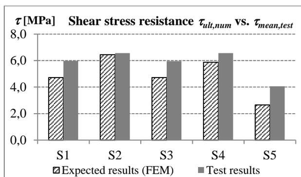
Fig. 11 Comparison of shear resistances (expected values and obtained values from the loading tests)
