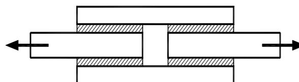
Fig. 1 Scheme of tested adhesively bonded joints
