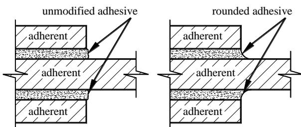
Fig. 6 Illustration of the adhesive modification
