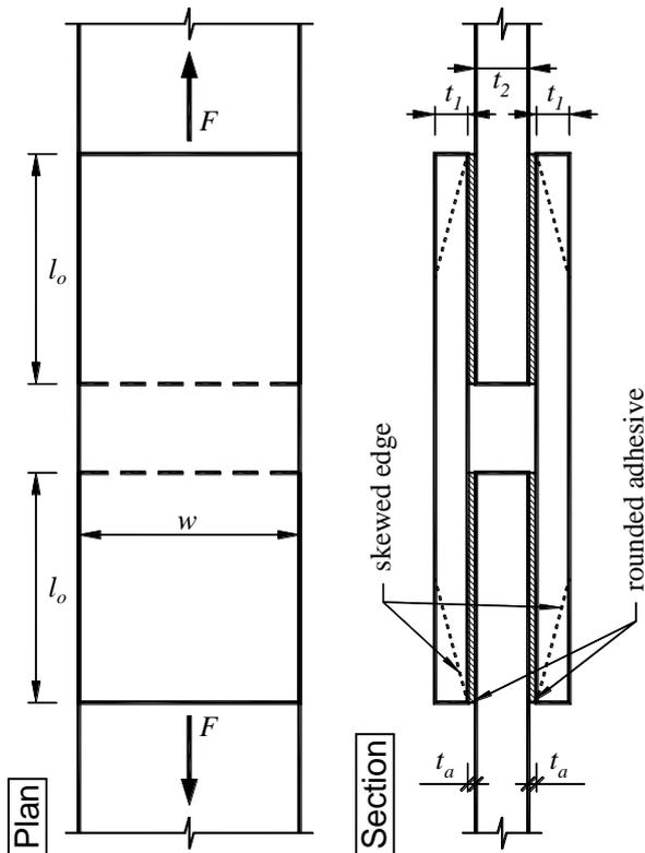
Fig. 5 Geometry and parameters of the tested adhesively bonded connection specimens
