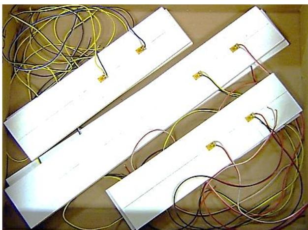
Fig. 2 Prepared specimens with the strain gauges
