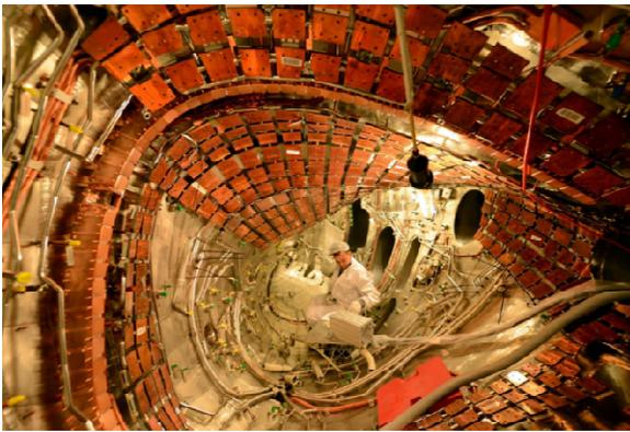
Fig. 2: internal view of Plasma Vessel with basic types of Plasma Facing Components (PFCs).
