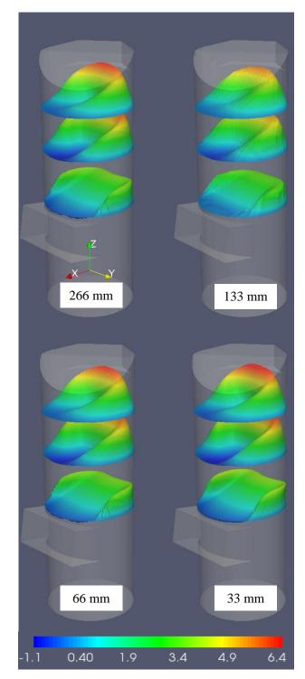
**Fig. 10** – Velocity fields (CFD) – z-velocity (m/s) for meshes with different element size
