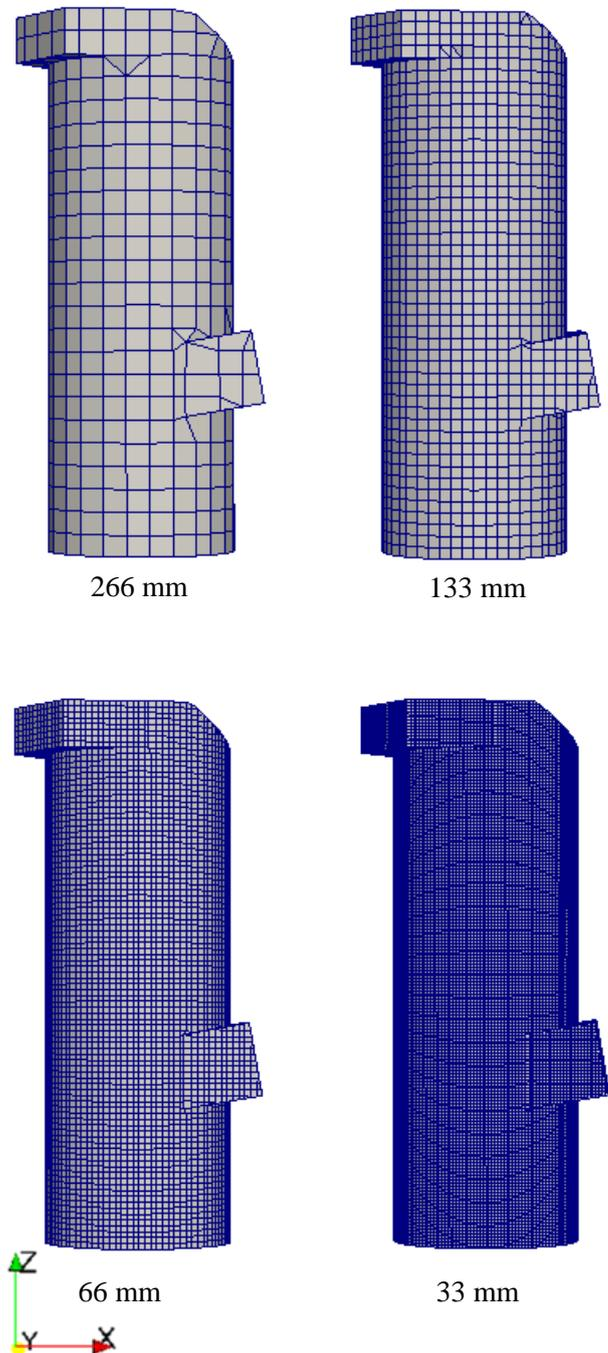
Fig. 8 – Computational meshes labeled by different element size
