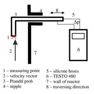
Fig. 6 – Block scheme of experimental setup
