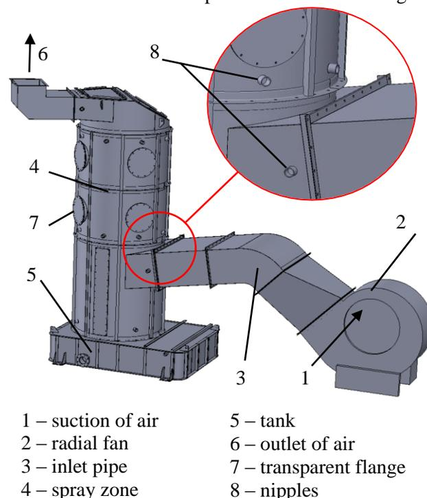
**Fig. 2** Assembly of reactor and fan – CAD model
