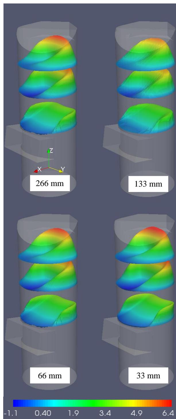
**Fig. 10** – Velocity fields (CFD) – z-velocity (m/s) for meshes with different element size
