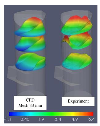
Fig. 11 – Velocity (comparison) – z-velocity (m/s)
