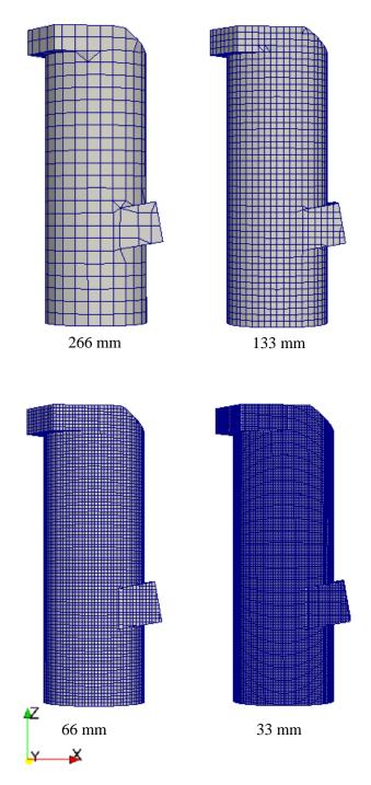
**Fig. 8** – Computational meshes labeled by different element size
