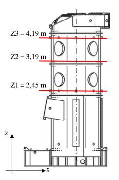
Fig. 4 – Reactor – Position of section planes
