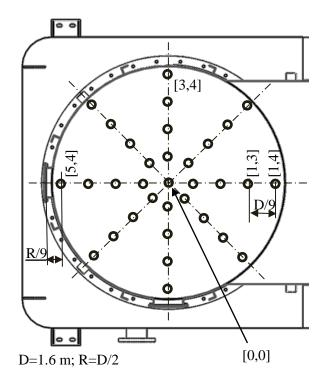
Fig. 5 – Measuring points – scheme and labeling
