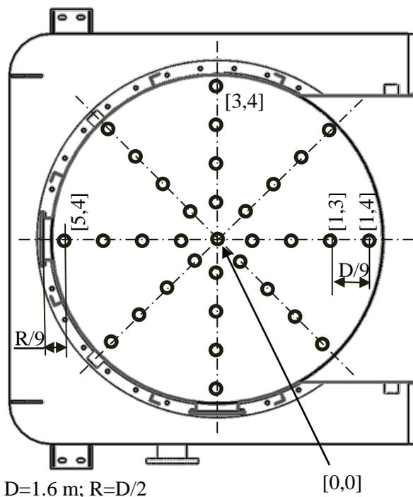
Fig. 5 – Measuring points – scheme and labeling
