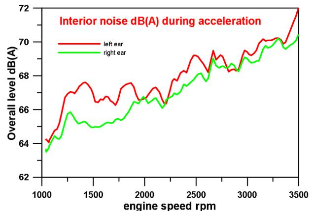
Fig. 3: Overall noise level in dB(A) vs. RPM (left ear: red curve, right ear: green curve).
