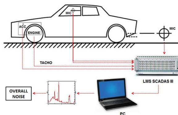
Fig. 1: Noise and vibration experimental setup.
