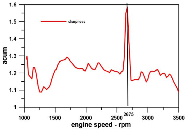
Fig. 4: Sharpness vs. RPM.
