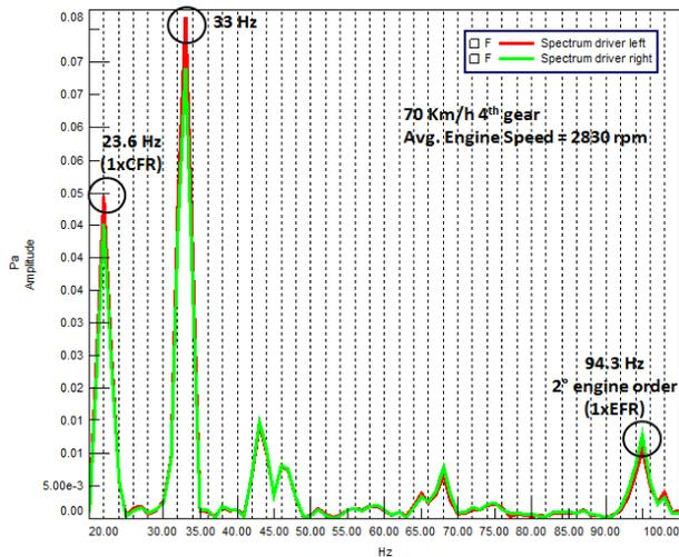
Fig. 6: Left and right driver noise frequency spectra @ 70 Km/h – 4<sup>th</sup> gear condition.
