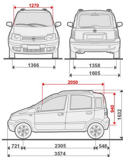
Fig. 9: Dimensions expressed in millimeters of vehicle under test.
