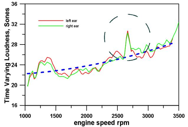
Fig. 2: Main engine parameters and Time Varying Loudness vs. RPM during vehicle acceleration.
