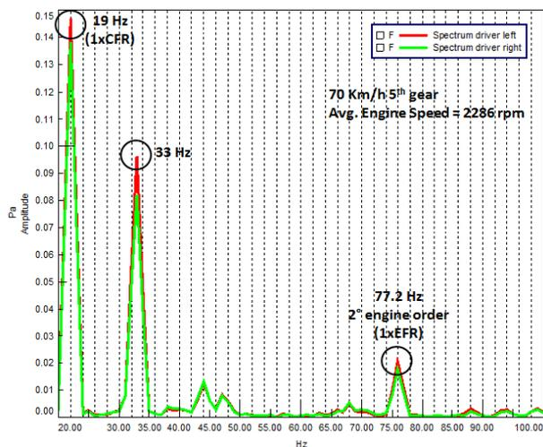
Fig. 7: Left and right driver noise frequency spectra @ 70 Km/h – 5<sup>th</sup> gear condition.
