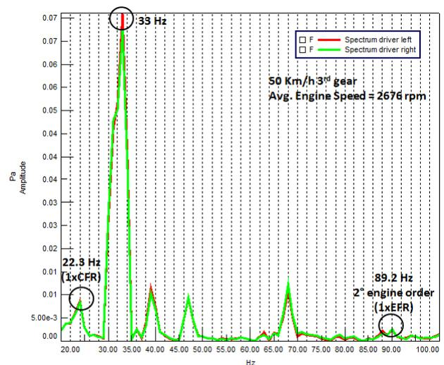
Fig. 5: Left and right driver noise frequency spectra @ 50 Km/h – 3<sup>rd</sup> gear condition.
