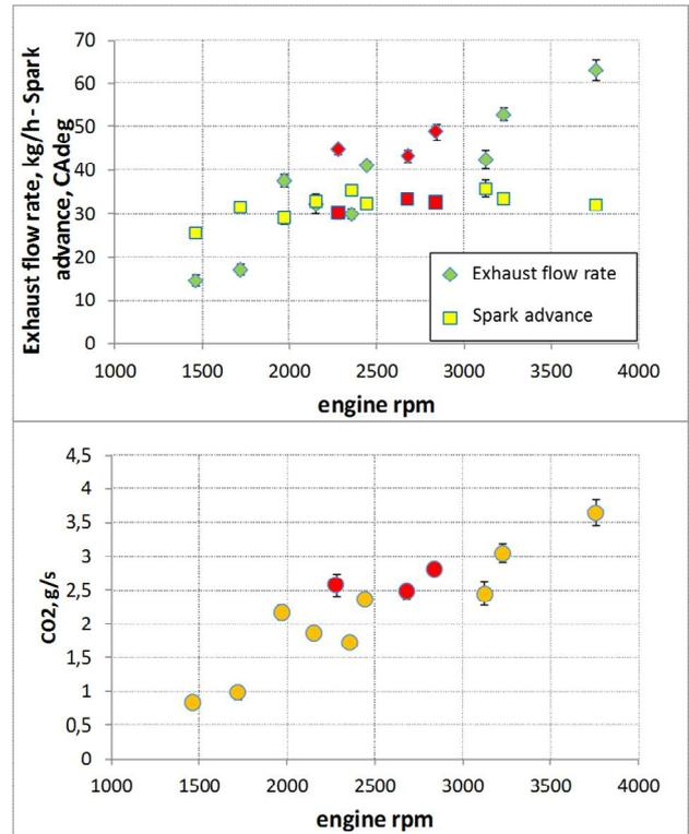
Fig. 8: Exhaust flow rate, spark advance and CO<sub>2</sub> emissions over the steady-states.
