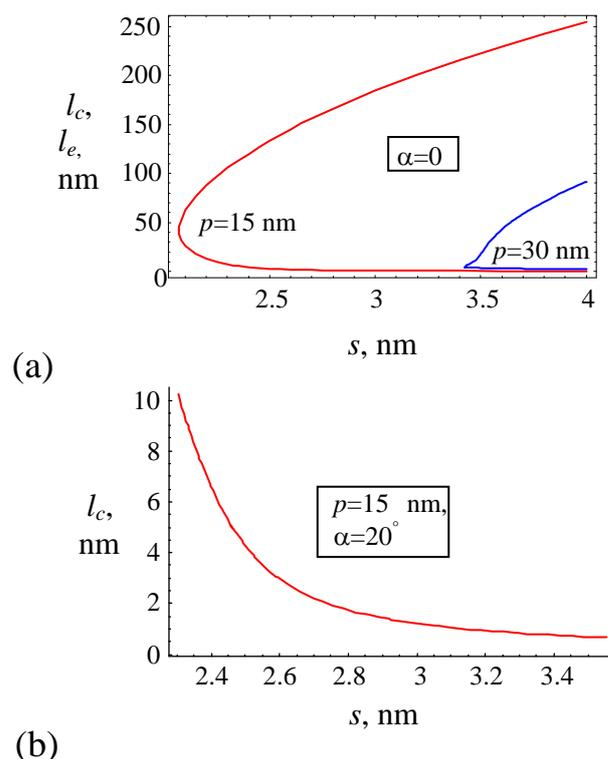
**Fig. 5.** Critical nanocrack length  $l_c$  (a,b) and equilibrium nanocrack length  $l_e$  (a) vs. twin boundary migration length  $s$ , for various values of the twin thickness  $p$  and angle  $\alpha$ .
