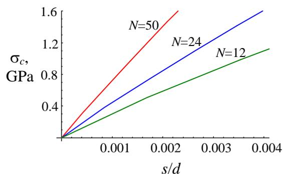
**Fig. 6.** Dependences of the critical applied load  $\sigma_c$  for collective twin boundary migration in a specified grain of nanotwinned Cu on the normalized twin boundary migration length  $s/d$ , for various numbers of twin boundaries.
