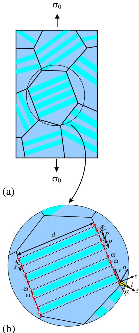
**Fig. 3.** Formation of a nanocrack in a deformed nanotwinned metallic solid. (a) Deformed nanotwinned metallic solid (general view). (b) Twin boundary migration in the grain is accompanied by the formation of an array of disclination quadrupoles and induces the generation of a nanocrack.
