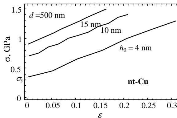
**Fig. 2.** Dependences of the flow stress  $\sigma$  on the plastic strain  $\varepsilon$  at various values of the initial (before plastic deformation) nanotwin thickness  $h_0 = 4$  nm, 10 nm and 15 nm.
