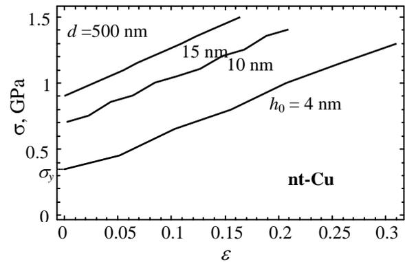
**Fig. 2.** Dependences of the flow stress  $\sigma$  on the plastic strain  $\varepsilon$  at various values of the initial (before plastic deformation) nanotwin thickness  $h_0 = 4$  nm, 10 nm and 15 nm.
