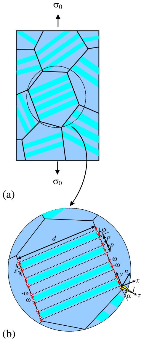
**Fig. 3.** Formation of a nanocrack in a deformed nanotwinned metallic solid. (a) Deformed nanotwinned metallic solid (general view). (b) Twin boundary migration in the grain is accompanied by the formation of an array of disclination quadrupoles and induces the generation of a nanocrack.
