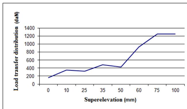
Fig.1: The load transfer distribution between wheels number 1 and number 2
