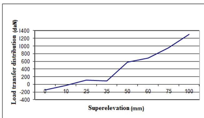
Fig.3: The load transfer distribution between wheels number 3 and number 4
