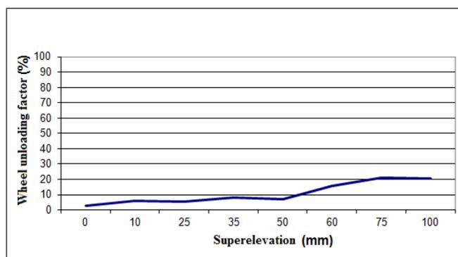
Fig.2: The wheel unloading factor for the wheel number 1
