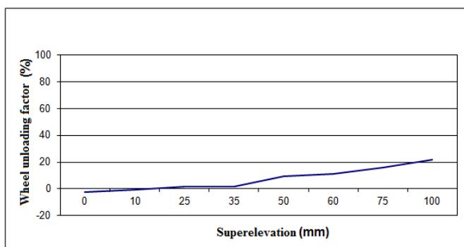
Fig.4: The wheel unloading factor for the wheel number 3
