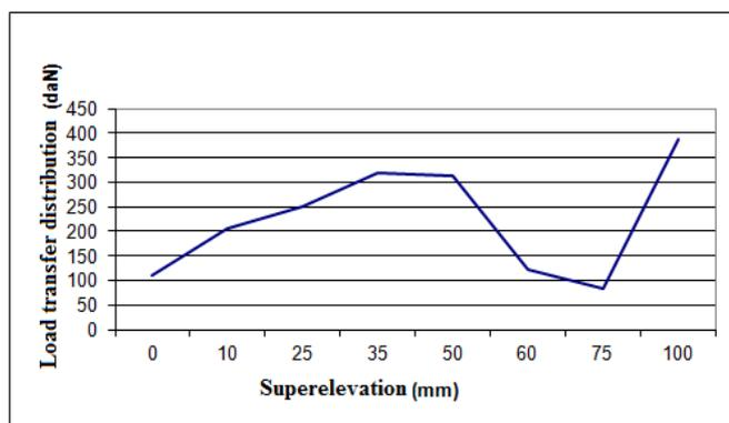
Fig.7: The load transfer distribution between wheels number 7 and number 8
