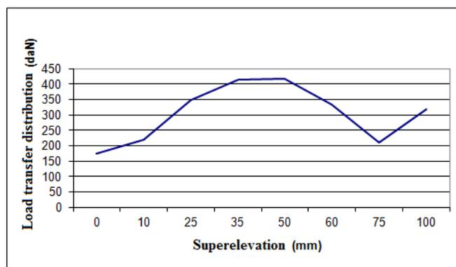
Fig.5: The load transfer distribution between wheels number 5 and number 6
