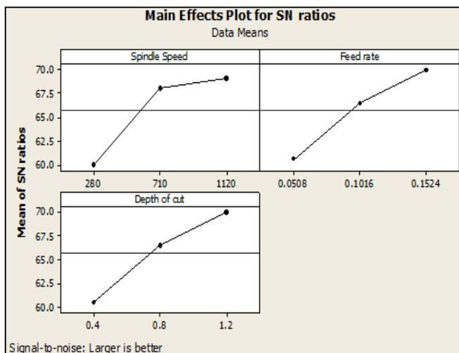
Fig. 1 Main effects plot for SN ratios of MRR
