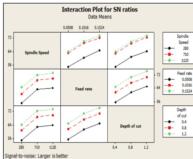
Fig. 2 Interaction plot for SN ratios of MRR
