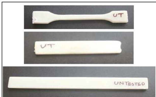
Fig. 3 Plain ABS test specimens
