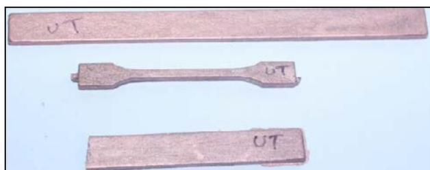
Fig. 4 Al reinforced ABS composites test specimens
