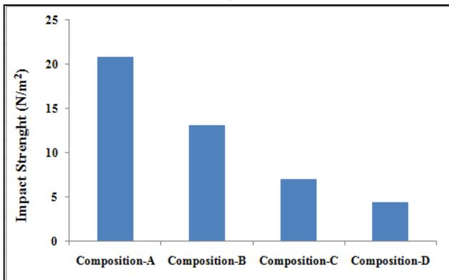
Fig. 8 Impact strength of unfilled ABS and ABS-Al composites
