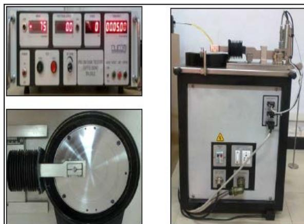
Fig. 5 Pin on disc tribometer
