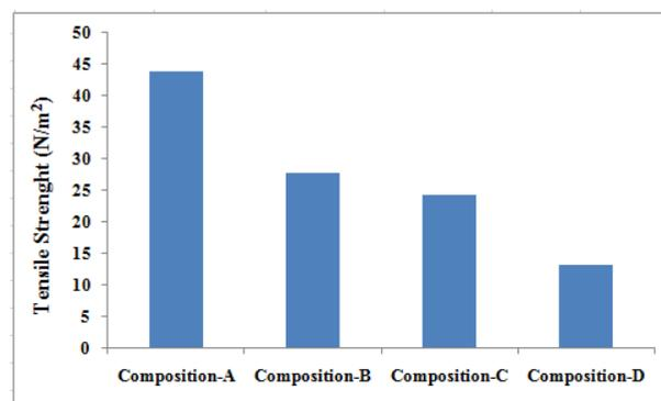
Fig. 6 Tensile strength of unfilled ABS and ABS-Al composites
