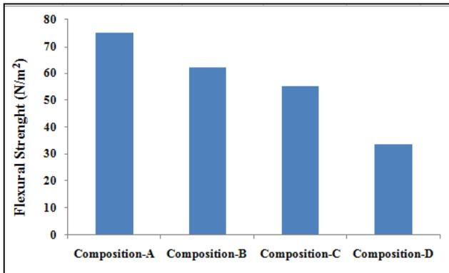
Fig. 7 Flexural strength of unfilled ABS and ABS-Al composites
