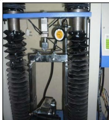
Fig. 1 b) Flexural test setup
