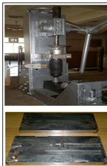
Fig. 2 Injection moulding machine with permanent die
