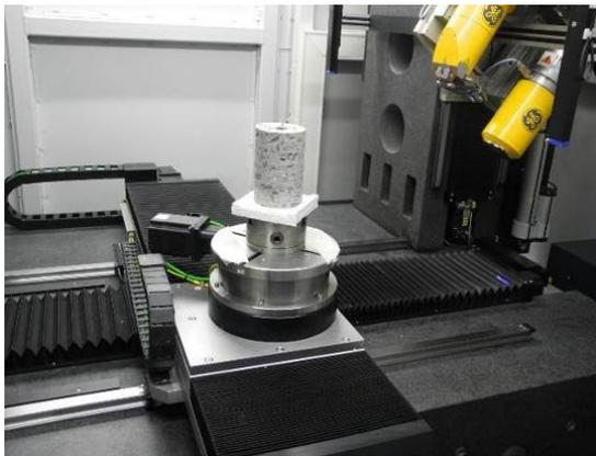
Figure 6: Tomograph GE phoenix,v|tome|x L 240 (top photo) and a cylindrical specimen fixed in its manipulator (bottom photo).
