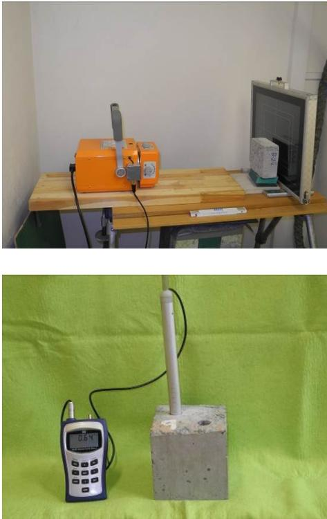
Figure 2: X-ray machine EcoRay HF 1040 with digital recording to PC equipment (top photo). PeMaSo-01 depth probe for magnetic measurements (bottom photo).
