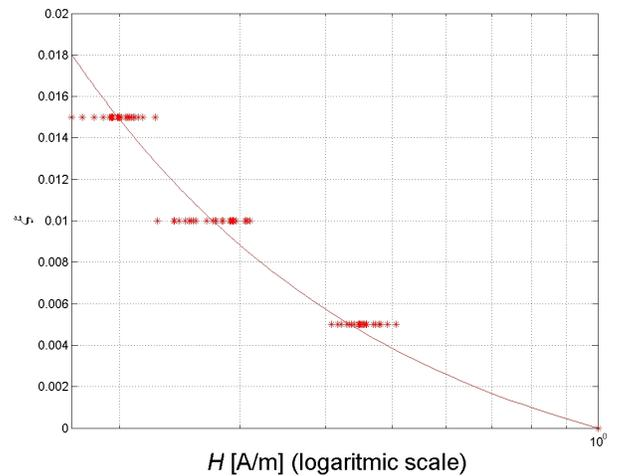
Figure 5: Application of the least squares technique to the identification of parameters  $\xi$  and  $\mu_s$  from magnetic measurements.
