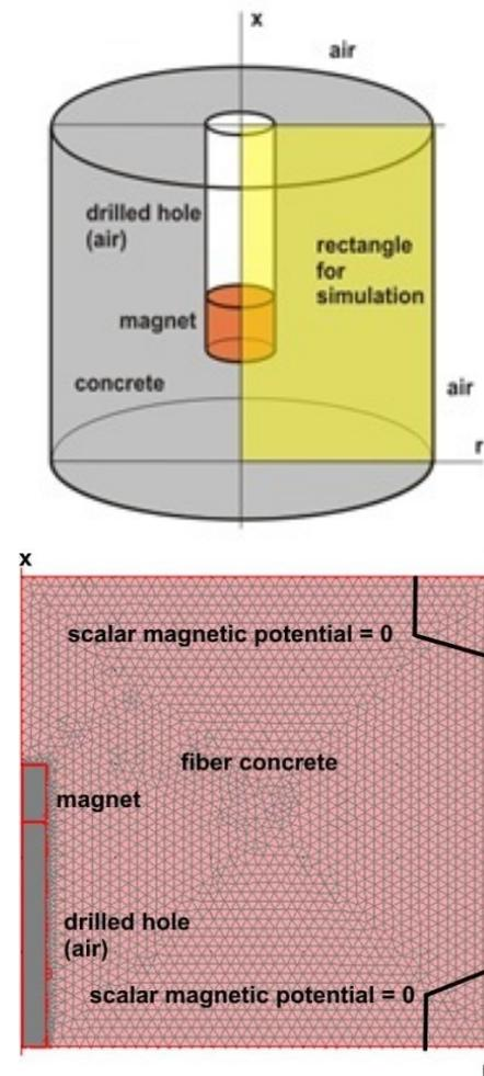
Figure 3: Radially symmetric geometrical arrangement of the magnetic experiment (top) and computational simplification, including finite/infinite element mesh (bottom).
