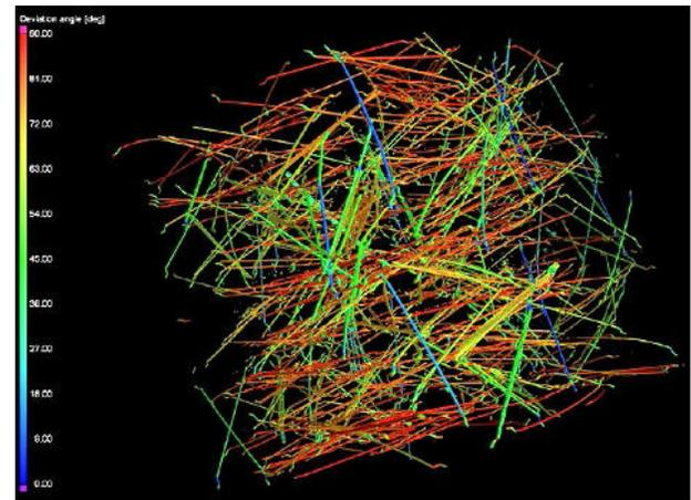
Figure 7: Cubic fibre concrete specimen, edge length 150 mm, required X-ray tube voltage 300 kV (images from the left to the right): axonometric view on its surface, axonometric view inside its structure, axonometric projection of separated fibres in the cube specimen.
