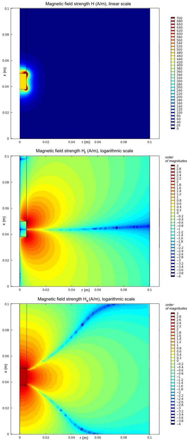
Figure 4: Results of COMSOL based on finite element simulation of stationary magnetic field strength.
