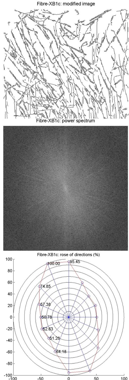
Figure 1: Evaluation of fibre orientation from the X-ray image (images from the top to bottom): original image, result of fibre localization, power spectrum  $P$ , resulting rose of fibre directions.
