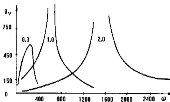
Fig. 14 Resonance curves for the vibration acceleration for three types of the membranes
