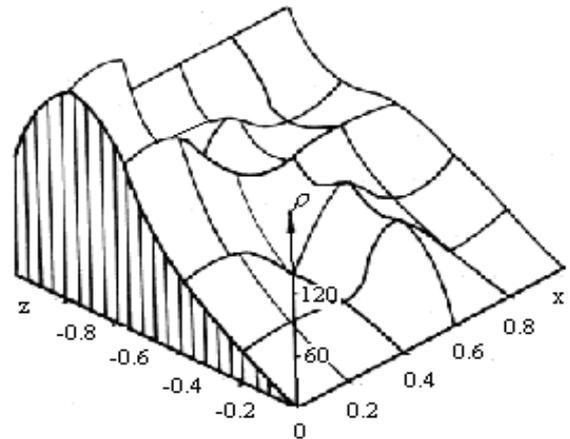
Fig. 24 Local abnormal density distribution due to abnormal heating in particle layer ( $Fo = 2 \cdot 10^{-5}$ )
