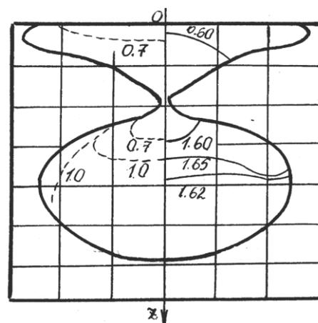
Fig. 6 Isobars and isotachs in a drop for  $b=0.4$
