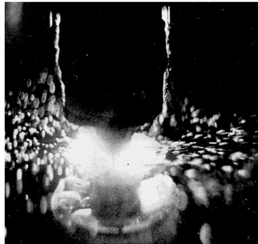
Fig. 15 Free film flow decay due to instability
