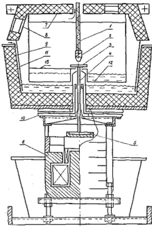
Fig. 13 The scheme of the Vibration type granulation film flow device with nitrogen atmosphere and liquid nitrogen coolant
