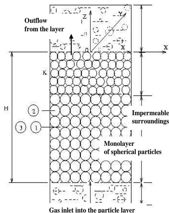
Fig. 21 Structural scheme of heterogeneous media
