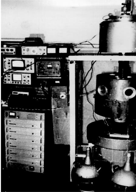
Fig. 12 Vibration film flow device with nitrogen atmosphere and liquid nitrogen coolant
