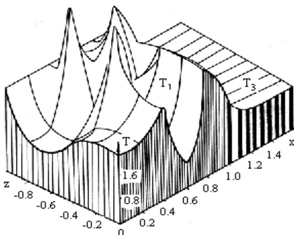
Fig. 23 Local abnormal heating in a particle layer with internal heat generation ( $Fo = 2 \cdot 10^{-5}$ )
