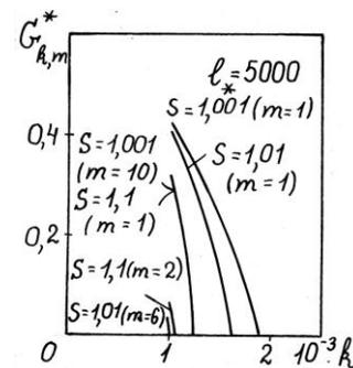
Fig. 4 Modified Bio numbers depending on the wave numbers and garnissage thickness.  $Pe=5000$
