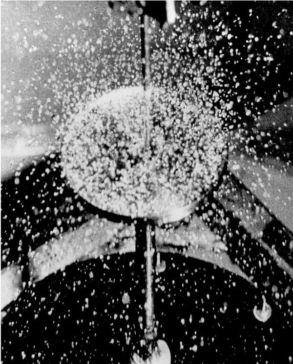
Fig. 17 Vibration controlled soliton-like film flow decay
