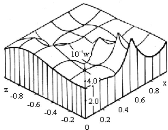
Fig. 25 Local abnormal filtration velocity due to abnormal heating in particle layer ( $Fo = 2 \cdot 10^{-5}$ )
