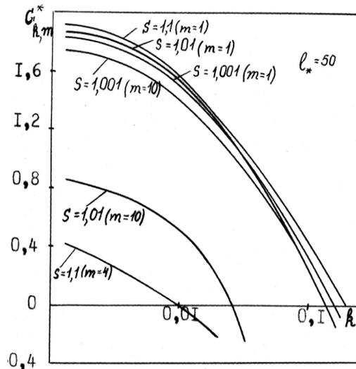
Fig. 3 Modified Bio numbers depending on the wave numbers and garnissage thickness.  $Pe=50$
