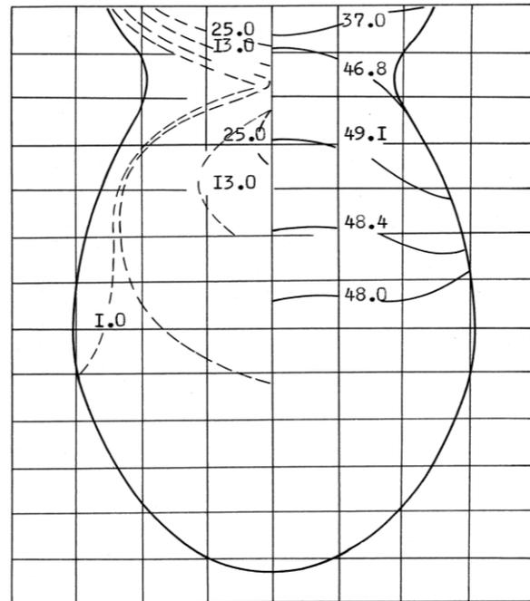
Fig. 5 Isobars and isotachs in a drop for  $b=40$
