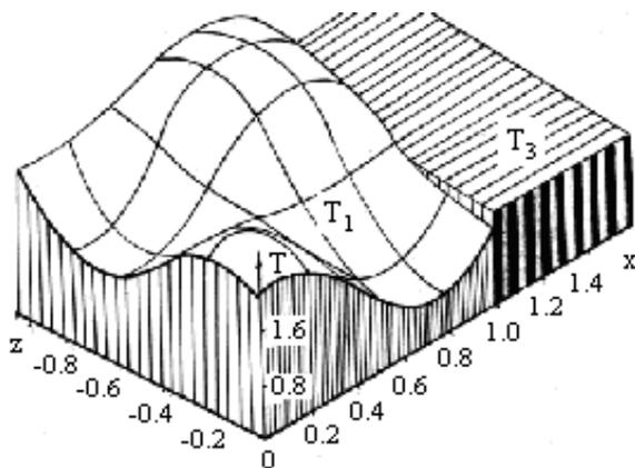
Fig. 22 Initial temperature perturbation in a steam flow  $T_1$  and surrounding  $T_3$  ( $Fo = 0$ ), computed by time step  $\Delta Fo = 2 \cdot 10^{-8}$ .
