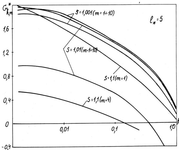
Fig. 2 Modified Bio numbers depending on the wave numbers and garnissage thickness.  $Pe=5$
