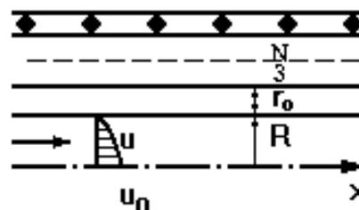
Fig.1 Flow in cylindrical channel with solidification on the wall with heat flux control system
