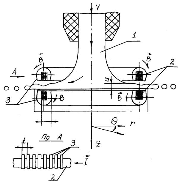
Fig. 9 Electromagnetic system for film flow decay
