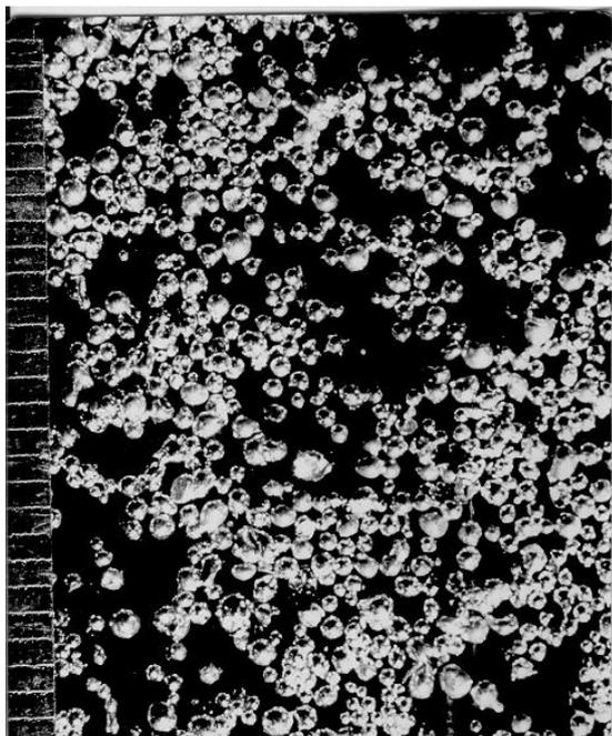
Fig. 18 Particles of metal produced in soliton-like regime on vibration type granulation machine
