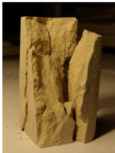
Fig. 5: The specimen after compression test. Typical brittle cracks are viewable on the specimen.
