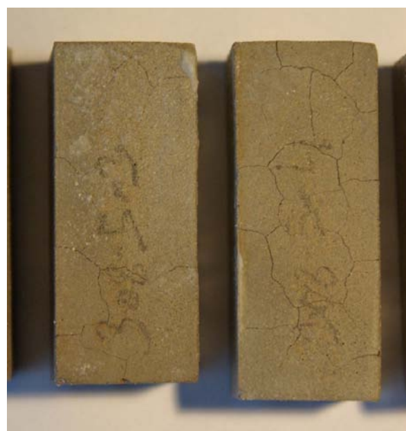
Fig. 2: Damage of specimens by temperature (600°C).
