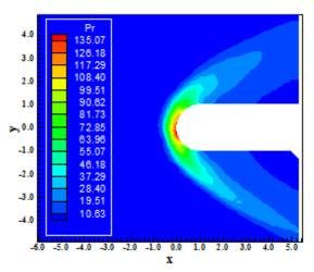
Fig. 21 Pressure contours.
