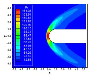
Fig. 16 Pressure contours.
