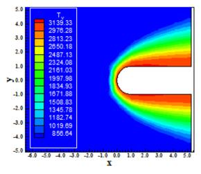
Fig. 14 Vibrational temperature contours.
