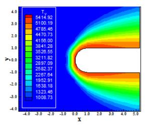
Fig. 4 Vibrational temperature contours.
