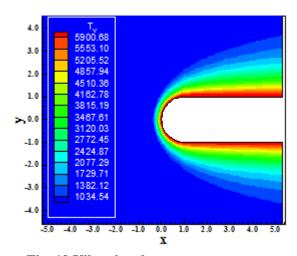
Fig. 19 Vibrational temperature contours.
