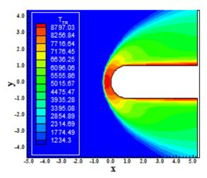
Fig. 8 T/R temperature contours.
