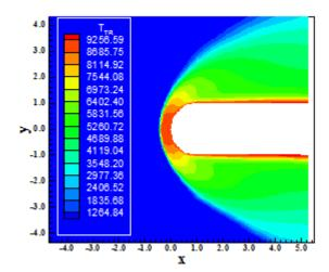
Fig. 28 T/R temperature contours.
