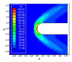
Fig. 11 Pressure contours.
