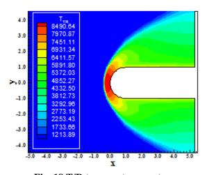
Fig. 18 T/R temperature contours.
