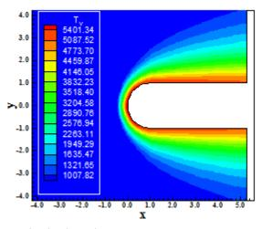
Fig. 9 Vibrational temperature contours.
