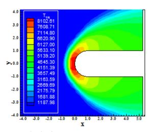
Fig. 3 T/R temperature contours.
