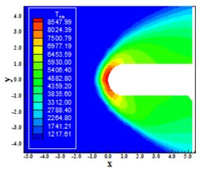
Fig. 23 T/R temperature contours.
