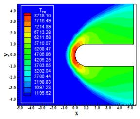
Fig. 13 T/R temperature contours.
