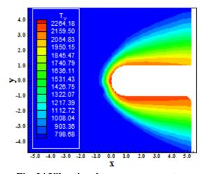
Fig. 24 Vibrational temperature contours.
