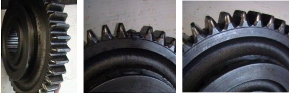
Fig.5: Healthy gear (left) – Broken gear (middle) - Worn tooth face gear (right)
