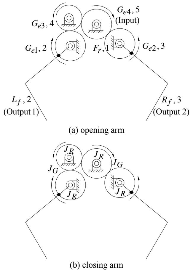
Figure 9 Schematic diagram of a new (5,7) robot arm
