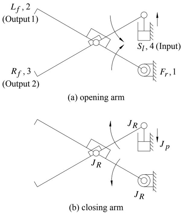
Figure 4 Schematic diagram of a (4,4) robot arm
