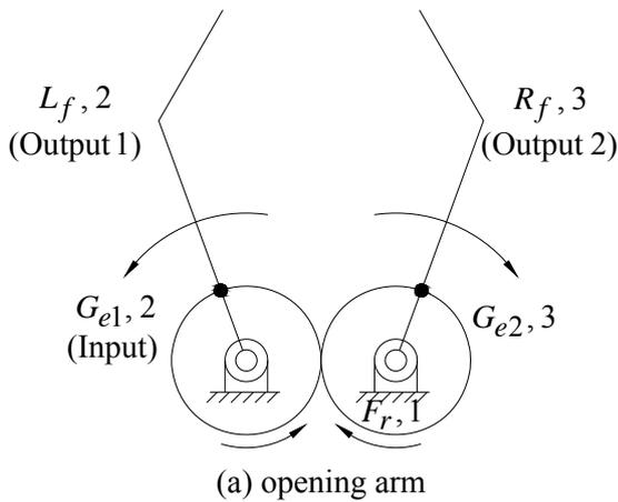
Figure 8 Schematic diagram of a (3,3) robot arm
