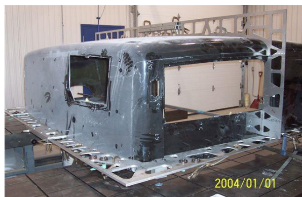
Fig.1 Inspection of non-rigid part using a jig - Source: Volvo, PREVOST Car
