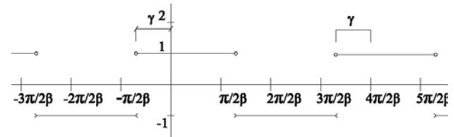
Fig. 2: The  $ang_y(\beta(x + \gamma))$  waveform.
