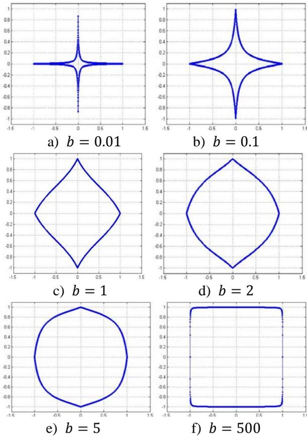
Fig. 13: different shapes of the function (48) for different values of  $b$  (presented in blue color).
