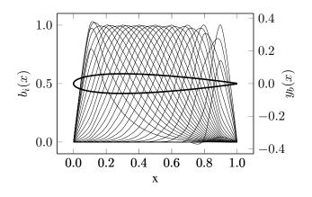
Figure 6: The baseline NACA0012 airfoil  $y_b(x)$  and the Hicks-Henne basis functions  $b_i(x)$ .
