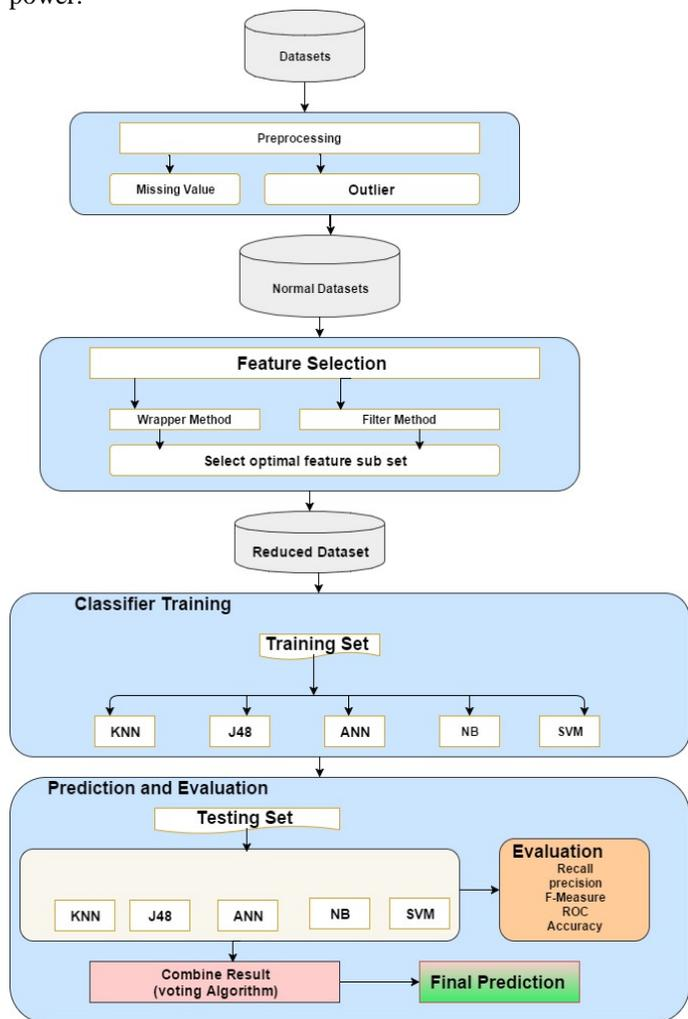
Fig 2. architecture of proposed ensemble model
