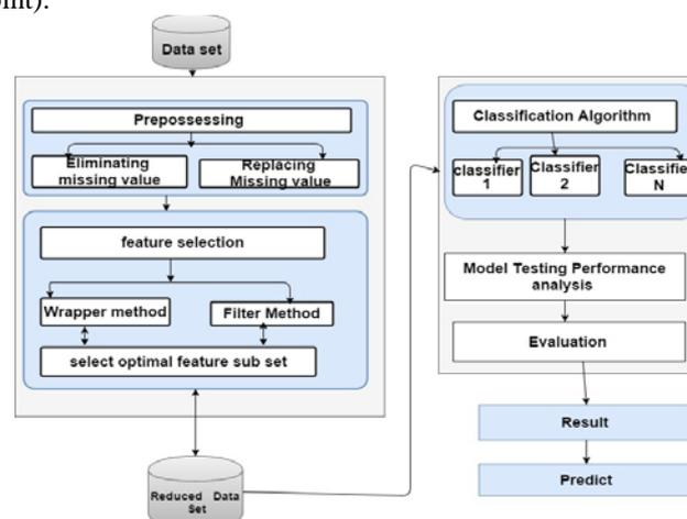
Fig. 1. system architecture for feature selection method
