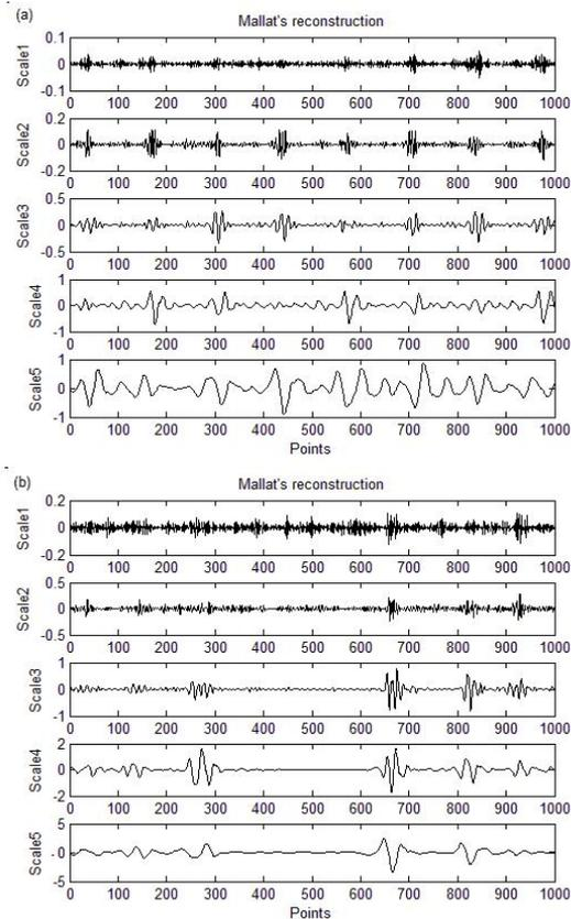
Fig.4 Examples of a segment of ECG signals: (a) represents the first five Scales of VF (b) represents the first five Scales of VT
