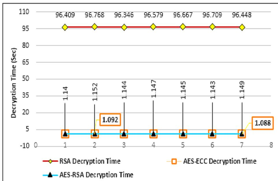
Figure 4: Decryption Time of Different Cryptosystems
