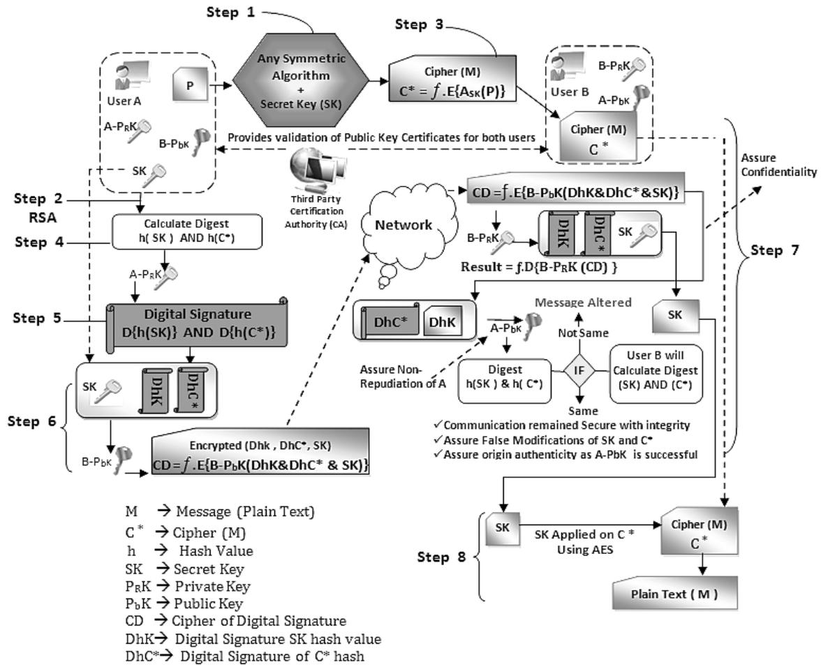
Figure 1: Generic Hybrid Encryption System (GHES) Framework
