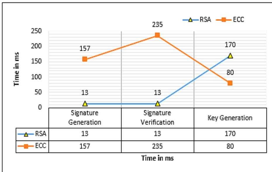
Figure 3: Key Generation, Signature Generation and verification Time
