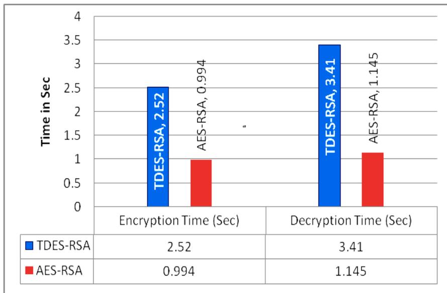
Figure 6: Encryption and Decryption time of TDES-RSA
