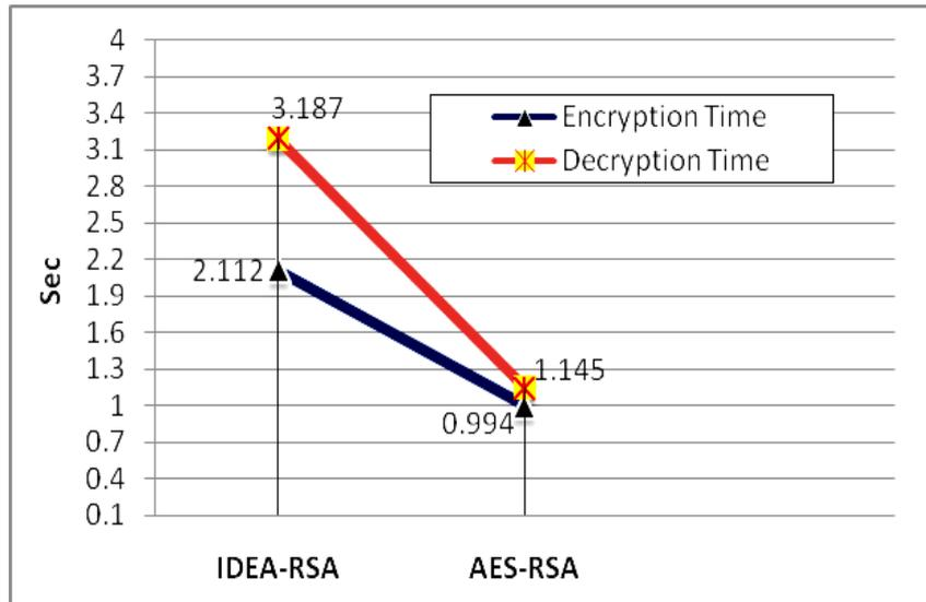
Figure 5: Encryptoin and Decryption time of IDEA-RSA
