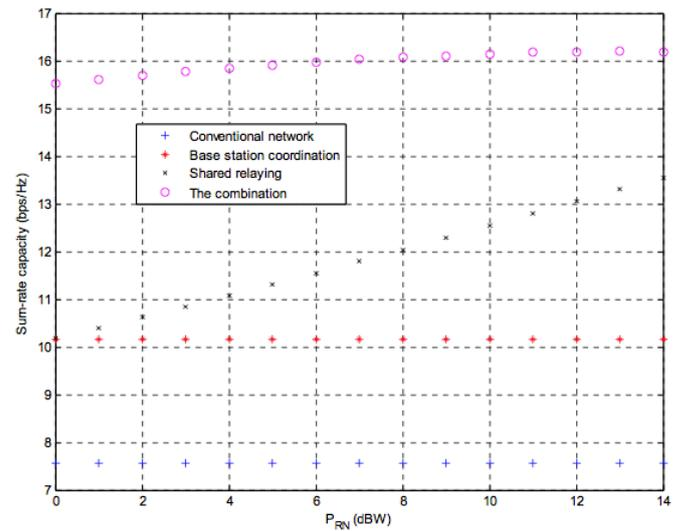
Fig. 5 Downlink sum-rate capacity versus  $P_{RN}$
