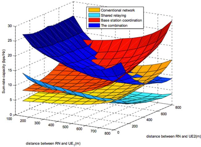
Fig. 8 Uplink sum-rate capacity versus distance apart from RN
