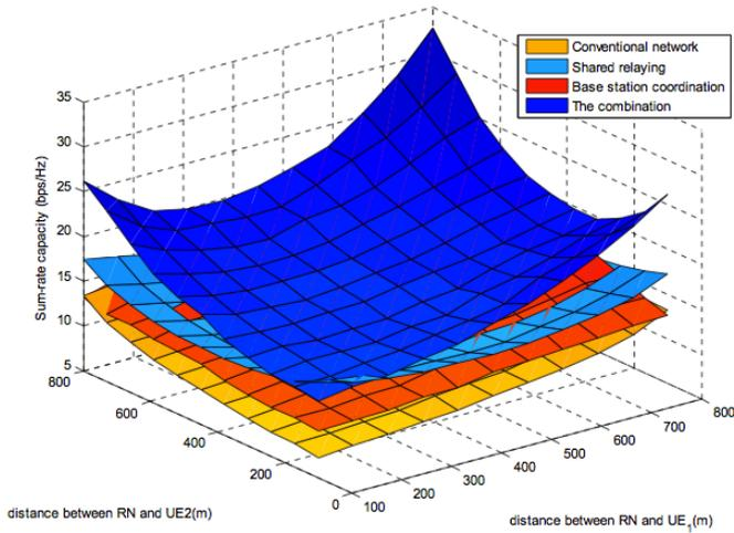
Fig. 7 Downlink sum-rate capacity versus distance apart from RN
