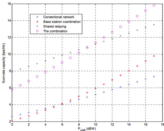
Fig. 3 Downlink sum-rate capacity versus  $P_{eNB}$
