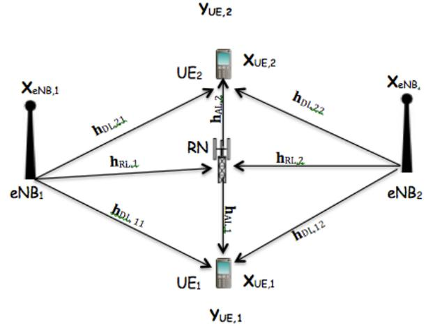
Fig. 2 Uplink (above) and Downlink (below) transmission in the combination scheme
