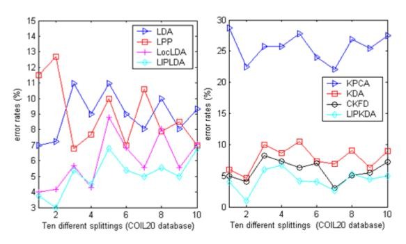
Fig.5 Comparison of eight DR methods in error rates on COIL20 database.
