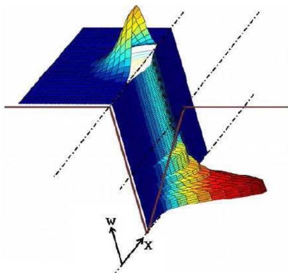
Fig.11. Solid (5182 Aluminum alloy) temperature field
