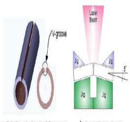
a Tube formed prior to welding process b Jig used in experiments
