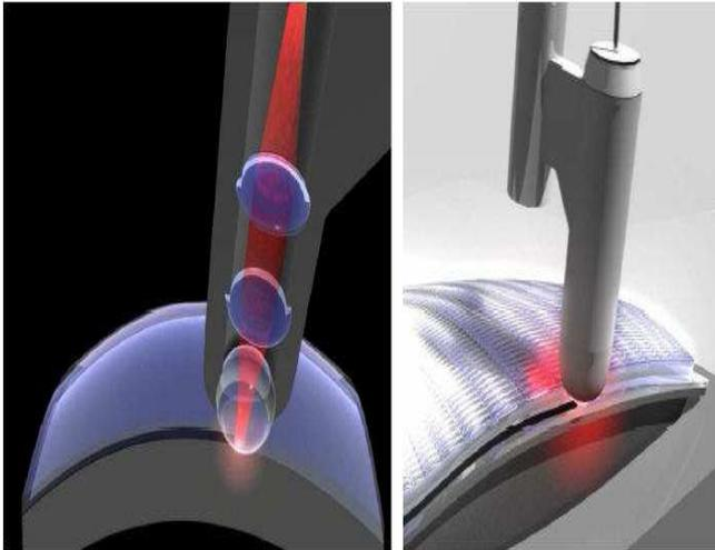
Fig.7. Schematic diagram of the welding technique
