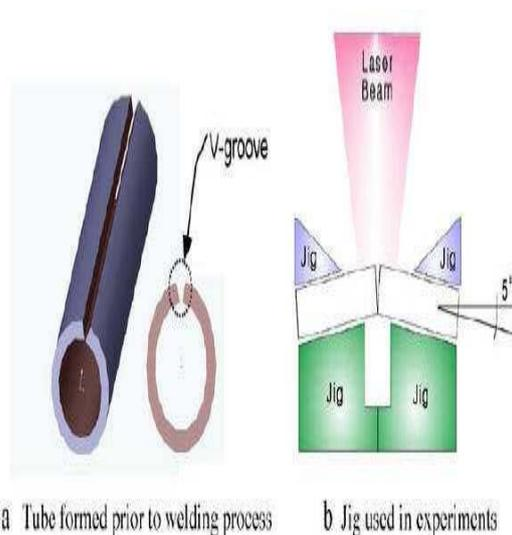
Fig.6. Joint shape and jig system used in experiments.
