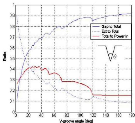
Fig.13. Absorbed power efficiency with respect to V-groove angle
