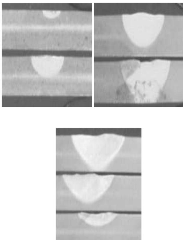
Fig.14. Conduction weld for 3mm gauge AA5083 using YAG laser ;Average power = 2000W ; Weld speed = 600mm/min
