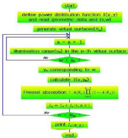
Fig. 8. Steps for the calculation of intensity functions
