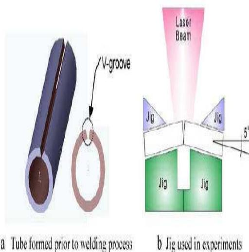
Fig.6. Joint shape and jig system used in experiments.
