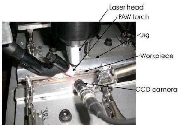
Fig.2. Experimental setup of laser system
