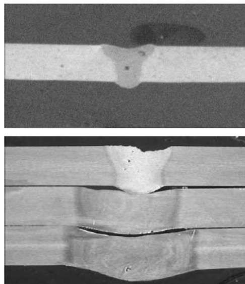
Fig.15 – (i) 3mm AA5083 LCW(YAG, Butt Weld),
