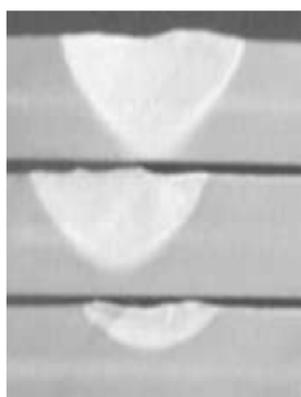
Fig.14. Conduction weld for 3mm gauge AA5083 using YAG laser ;Average power = 2000W ; Weld speed = 600mm/min
