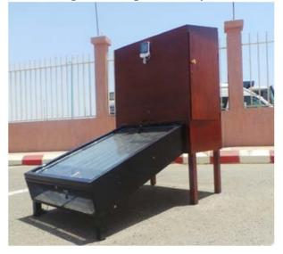
Fig. 2.1 Photo of the designed mixed-mode solar dryer
