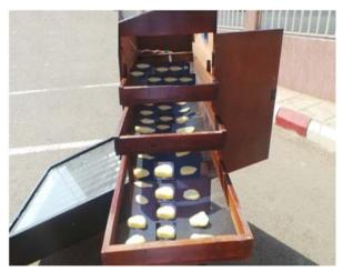
Fig. 2.3 Photo of the designed drying racks with freshly potato slides
