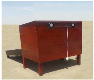
Fig. 2.4 Photo of the designed mixed-mode dryer from the bottom with two air blowers
