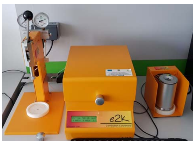
Fig. 5 Oxygen Bomb Calorimetric System and pressurized vessel
