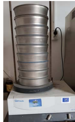
Fig. 2 Sieving machine used for separation of particles by size
