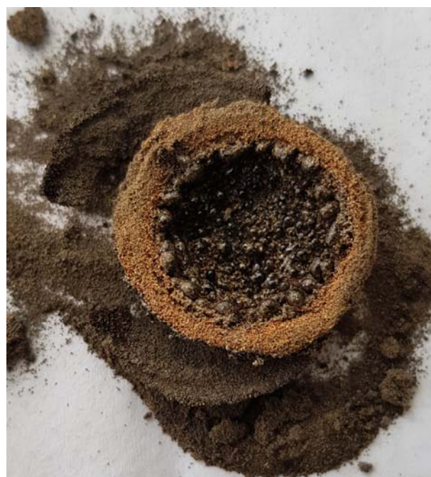
Fig. 8 Appearance of the ash sample after being subject to combustion with spiking material
