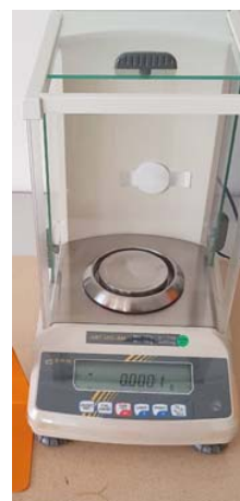
Fig. 6 Scale used for weighing the ash samples and calorimetric bomb vessel
