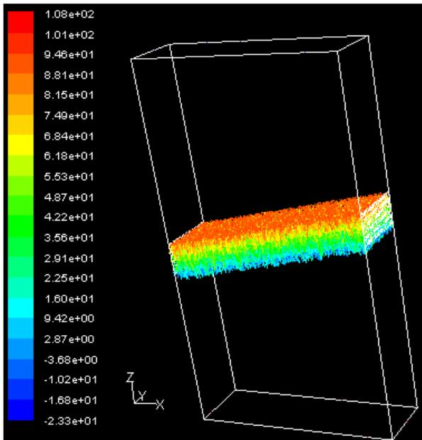
Figure 4. Velocity vectors colored by total pressure, Pa
