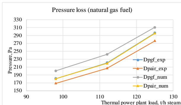
**Figure 7.** Pressure drop in the tract for natural gas running thermal power plant
