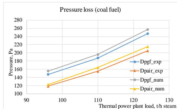
Figure 6. Pressure drop in the tract for coal running thermal power plant
