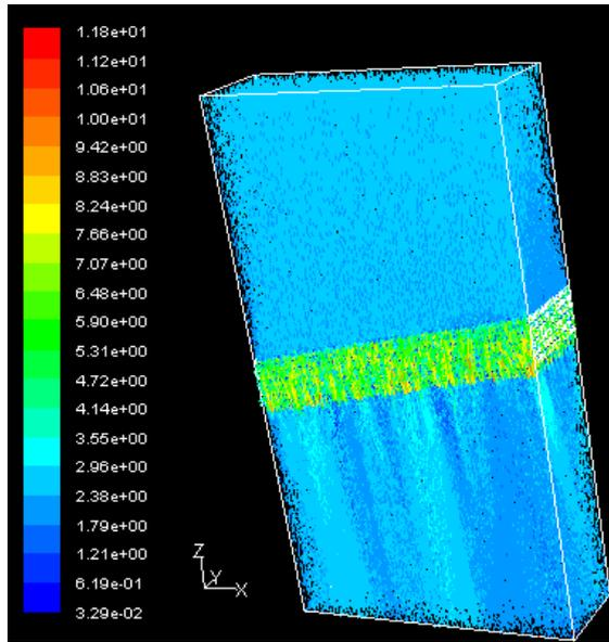
Figure 3. Flue gases velocity field distribution.
