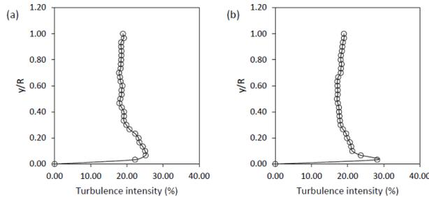
**Fig. 10.** Streamwise  $u'/\bar{U}$  distribution at (a) 13  $x/D$  (b) 63  $x/D$  for 15% WC after the pipeline constriction type GC 0.50.
