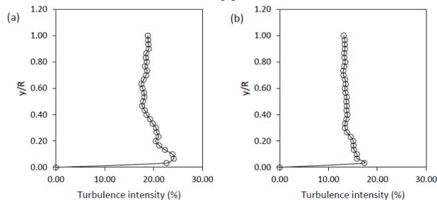
**Fig. 11.** Streamwise  $u'/\bar{U}$  distribution at (a) 13  $x/D$  (b) 63  $x/D$  for 20% WC after the pipeline constriction type GC 0.50.
