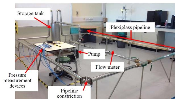
Fig. 1. Actual photo of the flow rig.
