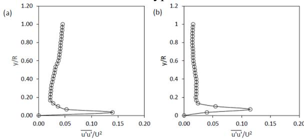
**Fig. 4.** The  $\overline{u'u'}/U^2$  profile at location (a)  $13 x/D$  and (b)  $63 x/D$  for 10% WC after the pipeline constriction type GC 0.50.
