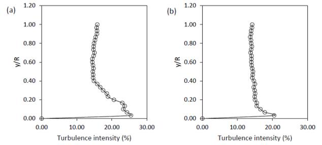
**Fig. 12.** Streamwise  $u'/\bar{U}$  distribution at (a) 13  $x/D$  (b) 63  $x/D$  for 25% WC after the pipeline constriction type GC 0.50.
