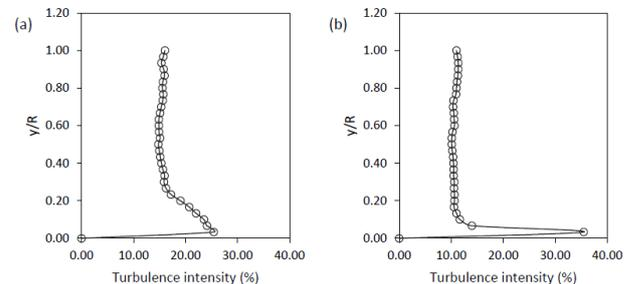
**Fig. 15.** Streamwise  $u'/\bar{U}$  distribution at (a) 13  $x/D$  (b) 63  $x/D$  for 40% WC after the pipeline constriction type GC 0.50.
