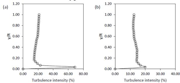
**Fig. 9.** Streamwise  $u'/\bar{U}$  distribution at (a) 13  $x/D$  (b) 63  $x/D$  for 10% WC after the pipeline constriction type GC 0.50.
