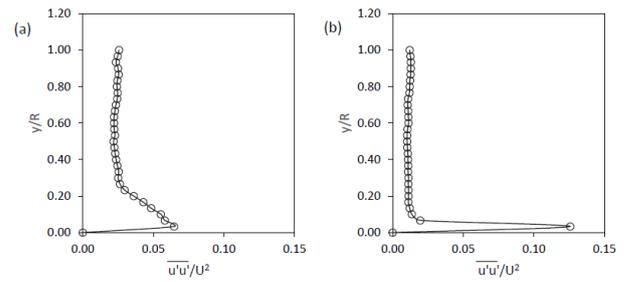
**Fig. 7.** The  $\overline{u'u'}/U^2$  profile at location (a)  $13 x/D$  and (b)  $63 x/D$  for 40% WC after the pipeline constriction type GC 0.50.
