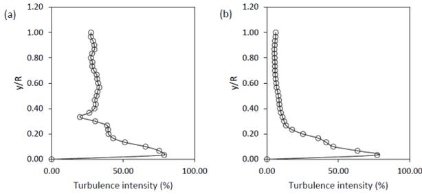
**Fig. 8.** Streamwise  $u'/\bar{U}$  distribution at (a) 13  $x/D$  (b) 63  $x/D$  for 0% WC after the pipeline constriction type GC 0.50.
