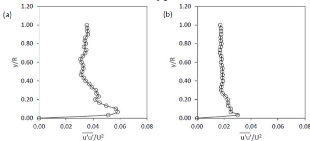
**Fig. 5.** The  $\overline{u'u'}/U^2$  profile at location (a)  $13 x/D$  and (b)  $63 x/D$  for 20% WC after the pipeline constriction type GC 0.50.
