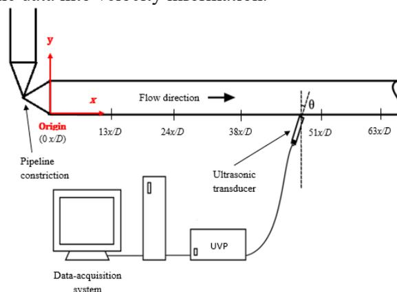
Fig. 2. Schematic diagram of the experimental setup for velocity measurement.
