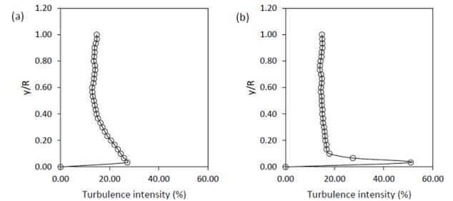
**Fig. 13.** Streamwise  $u'/\bar{U}$  distribution at (a) 13  $x/D$  (b) 63  $x/D$  for 30% WC after the pipeline constriction type GC 0.50.
