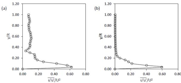
**Fig. 3.** The  $\overline{u'u'}/U^2$  profile at location (a)  $13 x/D$  and (b)  $63 x/D$  for pure crude after the pipeline constriction type GC 0.50.
