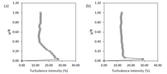
**Fig. 14.** Streamwise  $u'/\bar{U}$  distribution at (a) 13  $x/D$  (b) 63  $x/D$  for 35% WC after the pipeline constriction type GC 0.50.
