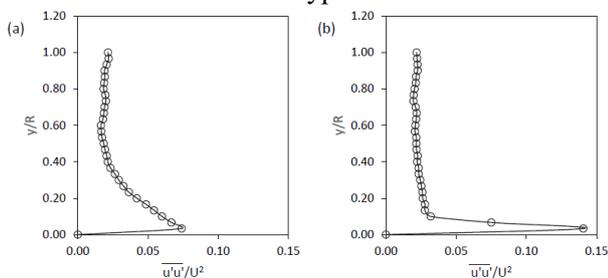
**Fig. 6.** The  $\overline{u'u'}/U^2$  profile at location (a)  $13 x/D$  and (b)  $63 x/D$  for 30% WC after the pipeline constriction type GC 0.50.
