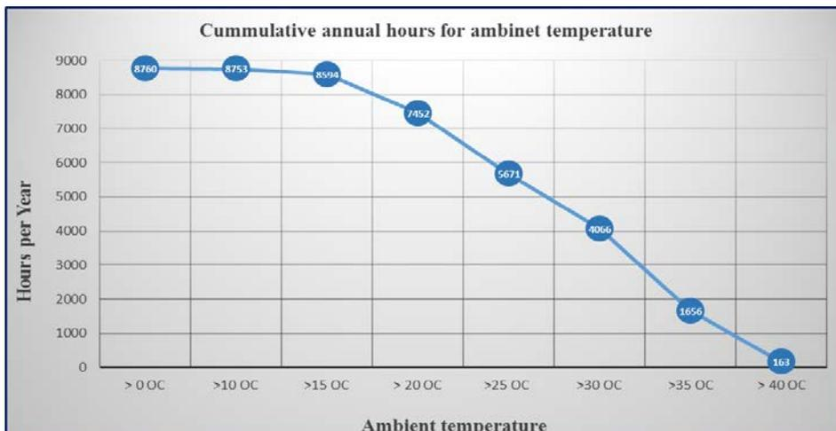
Figure (3) Cumulative annual hours for ambient temperature
