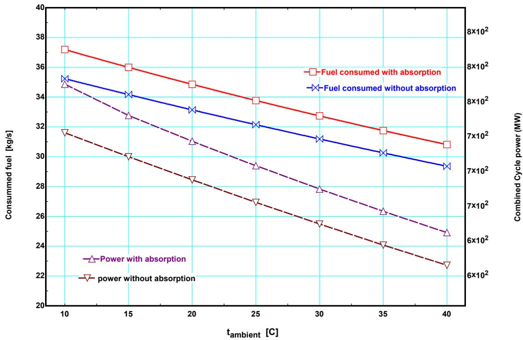
Figure (5) Effect of ambient temperature on fuel and power generated with and without GTIAC
