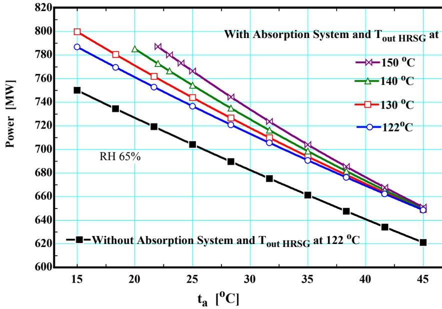
Figure (4) Effect of ambient air temperature on the plant generated power
