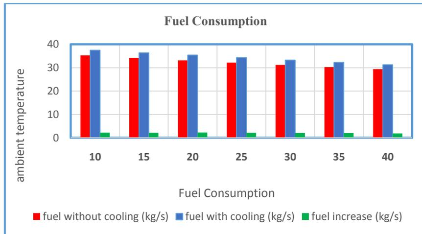
Figure (6) Change of Fuel Consumption Due to GTIAC
