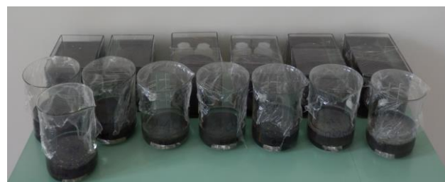
Fig.1 Settlement samples during alkali test
