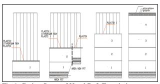
Fig 4. Curing Stage of Hotel Raft Foundation
