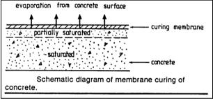
Fig 1. Curing method in maintaining temperature
