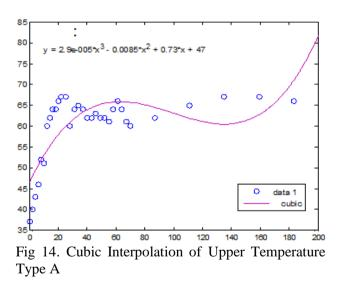
It can be seen from figure 14-17, simple interpolation approach using cubic spline method in predicting temperature development during specified time. From type A-D, each type similar behavior that the constant for third degree is significantly small. Therefore, second degree polynomial can be used as starting approach model, with limited consideration, since it is needed complete parameters to determine precise and accurate behavior of temperature development in mass concrete construction.
