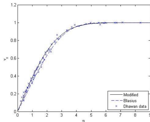
Figure 16. Predicted velocity profile (70) compared with experimental data of Dhawan [75].
