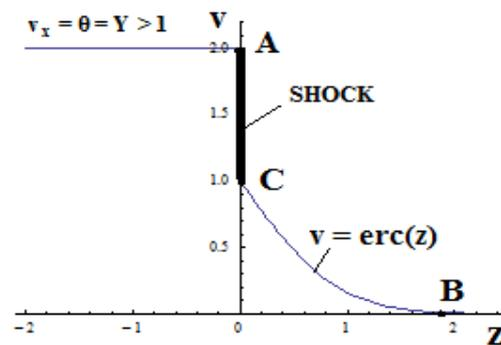
**Fig. 14 Structure of shock in polyatomic gas with thin and thick layers corresponding to type C shock structure of Taniguchi et al., [68].**
