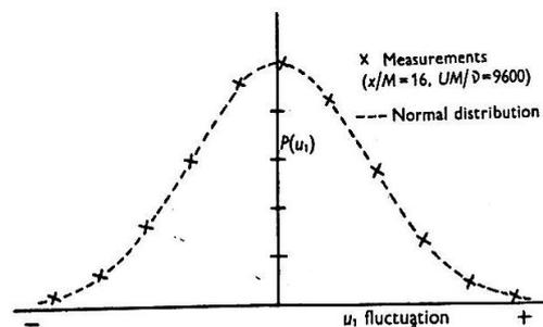
**Fig. 5** Measured velocity distribution in isotropic turbulent flow by *Townsend* [45].
