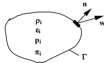
**Fig. 21 Conservation of  $(\rho_i, \epsilon_i, p_i, \pi_i)$  in an arbitrary domain  $\Gamma$  with unit outward normal  $\mathbf{n}$ .**
