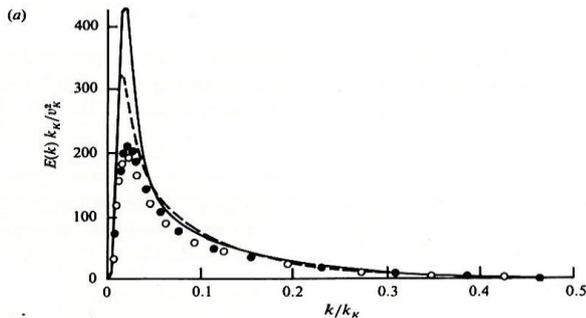
**Fig. 8 Normalized three-dimensional energy spectra for isotropic turbulence [48].**
