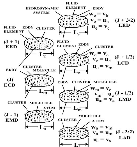
**Fig. 2 Hierarchy of statistical fields for equilibrium eddy-, cluster-, and molecular-dynamic scales and the associated laminar flow fields.**
