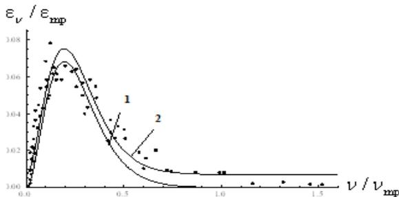
**Fig. 9 One-dimensional dissipation spectrum [51] compared with (1) *Planck* energy distribution (2) *Planck* energy distribution with constant displacement.**
