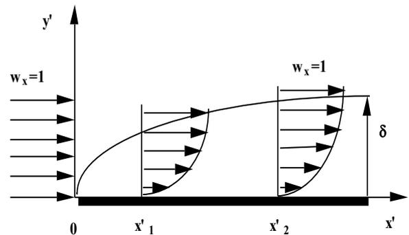
Fig. 15 Laminar boundary layer over a flat plate.
