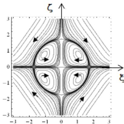
Fig. 19 Flow field within liquid droplet at the stagnation point of viscous counter flow [92].
