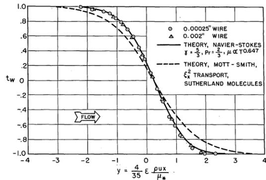
Fig. 13a Comparison between experiment and theory from Sherman [63] for normal shock in helium at  $Ma = 1.82$ .
