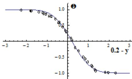
**Fig. 13b Comparison between measured normalized wire temperature  $\Theta$  versus position  $(0.2 - y)$  in normal shock [63] and theory (45).**
