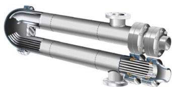
Fig. 7. Double pipe heat exchanger [7]
