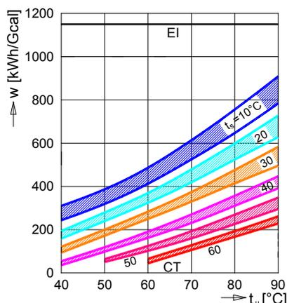
Fig. 2 Electricity consumption for the heat production
