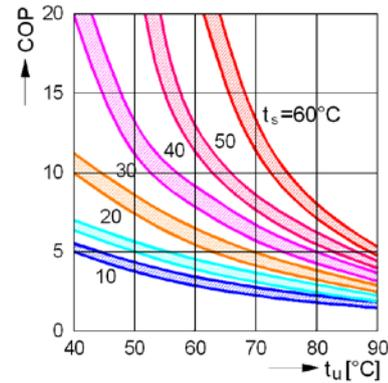
Fig. 1 Variation of heat pump efficiency
