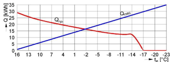
Fig. 5 Variation of heat requirement and HP thermal power with outdoor temperature
