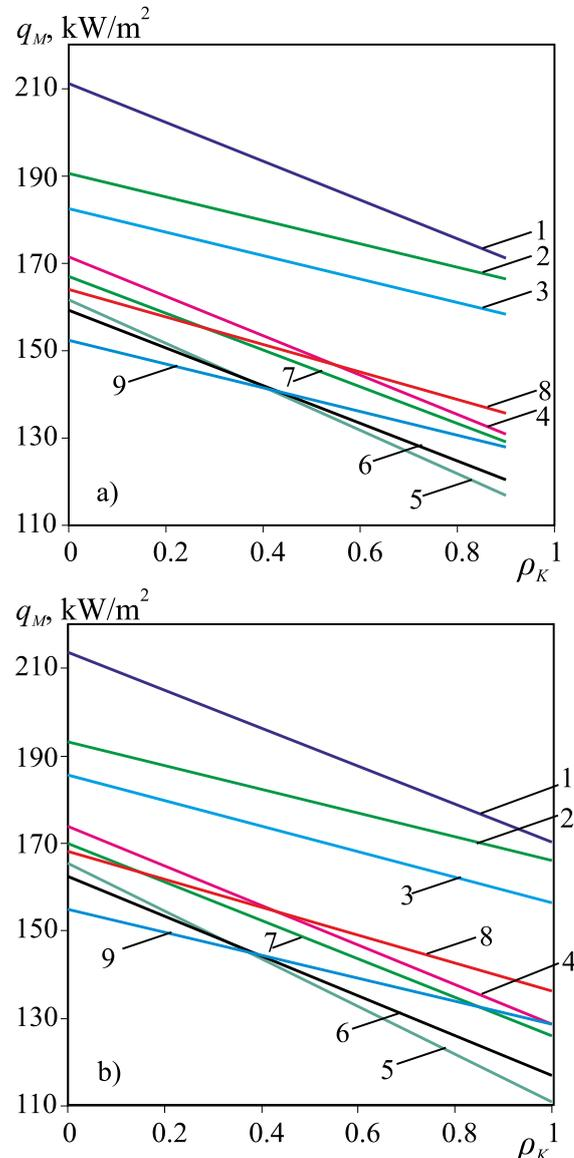
Fig.4. Dependence of resulting heat flux density  $q_M$  absorbed by receiving surface of flat layer of natural gas combustion products in dependence on reflectivity of adiabatic refractory surface  $\rho_K$ .
