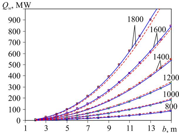
Fig. 2. Total heat flux  $Q_w$  absorbed by the receiving surfaces (walls) of the boiler or process furnace in dependence on combustion chamber width  $b$ . Solid lines – our calculations by Monte-Carlo procedure, dotted lines – by H. Kremer [31]. Zone method computations parameter – furnace gas temperature  $T_g$ , °C, is indicated near the curves. Number of computation zones  $N_{CZ}=1$ .  $O_2$  content in oxidant  $[O_2] = 100\%$ .
