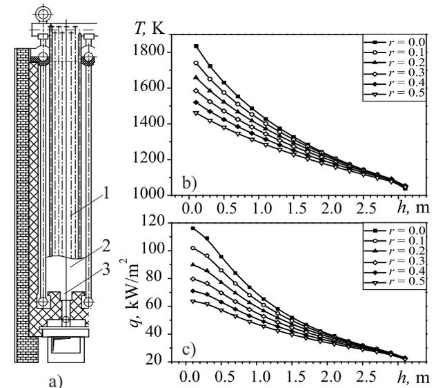
Fig. 7. Profiles of the combustion products temperature  $T$ , K (b) and the radiative heat fluxes  $q$ ,  $kW/m^2$  (c) by height of the boiler TVG-8 furnace (a) in dependence on mass recirculation ratio  $r$ .
