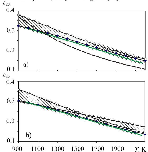
Fig. 1. Integral emissivity (blackness) factor of the combustion products  $\varepsilon_{CP}$  been calculated by means of various models.
