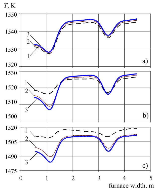
Fig. 10. Temperature profile of the billet across the furnace from the left edge to the axial longitudinal plane, in the exit cross-section plane of the furnace. Furnace output  $G_{fur}$ , t/h: a – 130, b – 150, c – 170. Steel emissivity factor  $\varepsilon_M = 0.9$ . Surfaces computation planes: 1 – upper; 2 – middle; 3 – lower.
