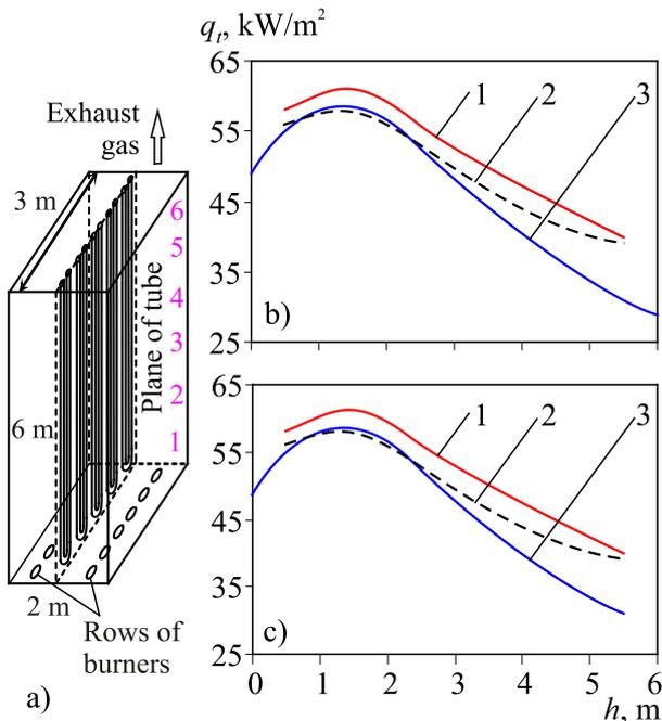
Fig. 6. Profile of resulting heat flux density  $q_t$  by furnace height  $h$  / Comparison of our original predicted data with earlier calculations.
