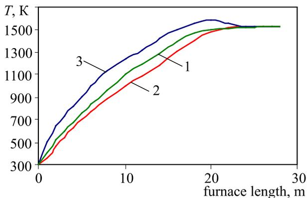
Fig. 9. Thermogram of the billet heating by the furnace length in the central longitudinal plane of the furnace (for middle cross-section by the slab's length).
