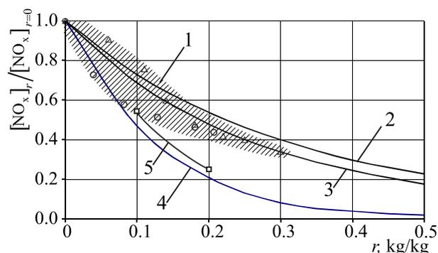
Fig. 11. Dependence of relative reduction of  $\text{NO}_x$  concentration on mass recirculation ratio  $r$  of the natural gas/air combustion products.
