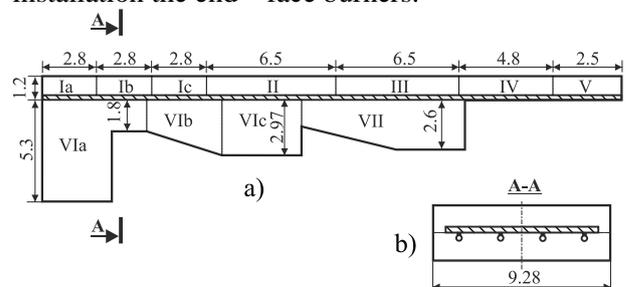
Fig. 8. The “DUNAFERR RT” Company's continuous pusher-type reheating furnace design (layout): a – longitudinal section; b – cross-section. The computation zones numbers are indicated with Roman figures.
