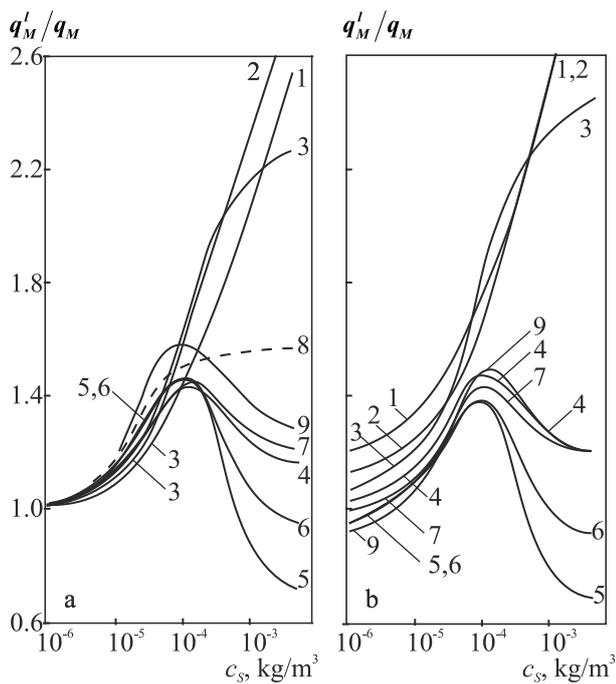
Fig.5. Relative value  $\bar{q}_{M,j}$  of specific resulting heat flux absorbed by receiver under liquid fuel combustion to that obtained by natural gas burning in dependence on soot concentration  $c_s$  ( $\text{kg/m}^3$ ) in combustion products.
