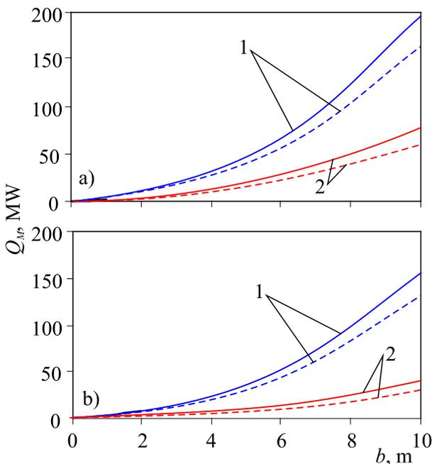
Fig. 3. Resulting total radiative heat flux  $Q_M$ , absorbed by ingot surface in the industrial furnace. Ingot temperature  $T_M$ , °C: a – 800; b – 1200. Furnace gases temperature  $T_g$ , °C: 1–1800; 2–1400; Solid lines – our calculations by Monte-Carlo procedure, dotted lines – by H. Kremer [31]. Number of computation zones  $N_{CZ}=1$ . Zone method computations parameter – furnace gas temperature  $T_g$ , °C.  $[O_2] = 21\%$  in oxidant.
