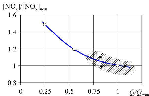
Fig. 12. Dependence of relative  $\text{NO}_x$  concentration  $[\text{NO}_x]/[\text{NO}_x]_{nom}$  on relative firing rate (load)  $Q/Q_{nom}$  of the boiler equipped with FIRB
