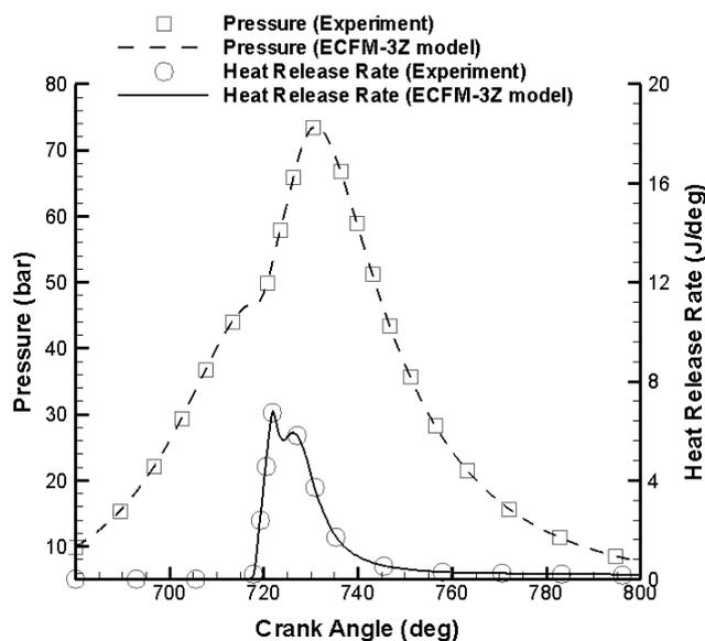
**Figure 2: Validation of pressure and heat release rates [17]**
