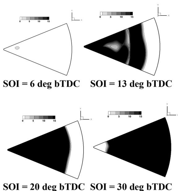
**Figure 19: Contours of NO<sub>x</sub> emissions (g/ kg of fuel) for different injection timing**
