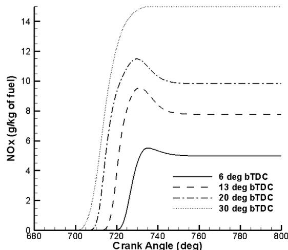
Figure 17: Nitrogen oxides at different injection timing
