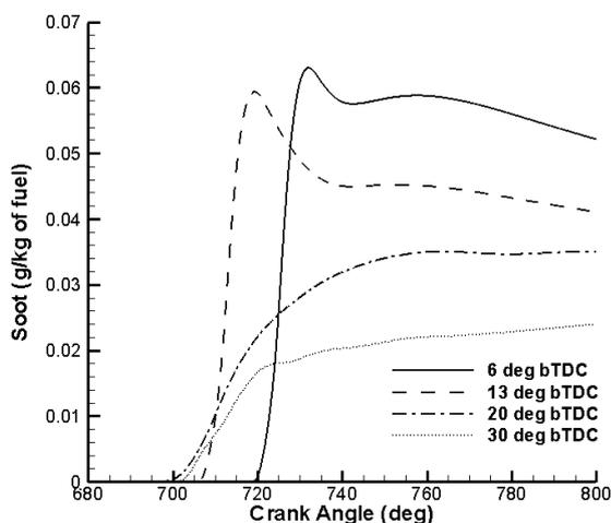
Figure 16: Soot distribution at different injection timing
