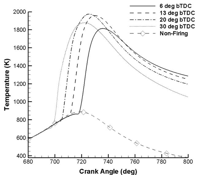
**Figure 10: Cylinder averaged temperature for various start of injection**
