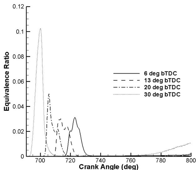
**Figure 20: Variation of equivalence ratio in the piston bowl at different Crank Angle**
