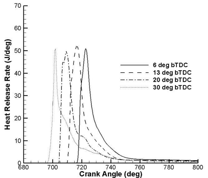
**Figure 9: Cylinder averaged heat release rate at different injection timing**
