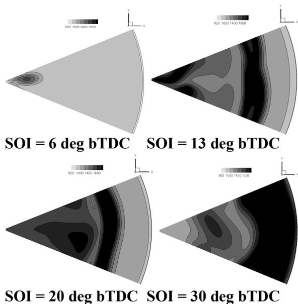
**Figure 13: Contours of temperature (K) for different injection timing**
