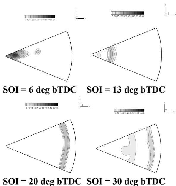
**Figure 14: Contours of flame surface density (1/m) for different injection timing**
