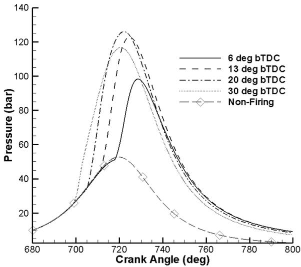
**Figure 8: Cylinder averaged pressure for firing and non-firing conditions at different start of injection**
