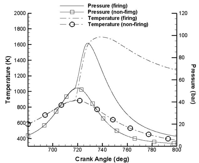
**Figure 7: Cylinder averaged pressure, temperature**
