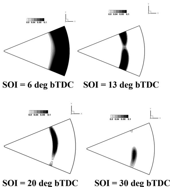
Figure 18: Contours of soot emissions (g/ kg of fuel) for different injection timing at TDC
