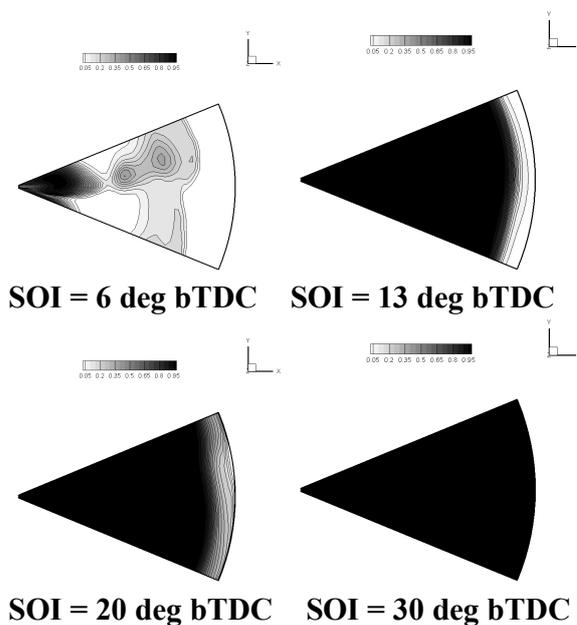
**Figure 15: Contours of progress reaction variable for different injection timing**
