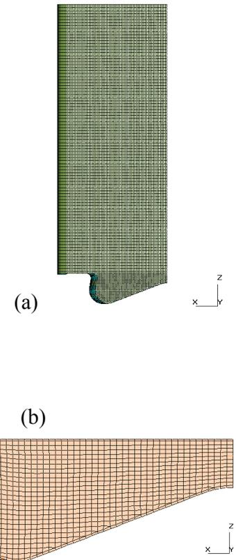
**Figure 1: Computational domain of engine cylinder at (a) 720 °CA and (b) 800 °CA**
