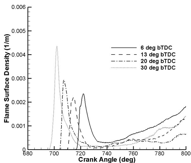
**Figure 12: Flame surface density at different injection timings**
