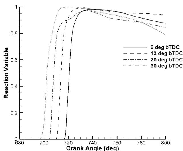
**Figure 11: Reaction variable for different injection timing**
